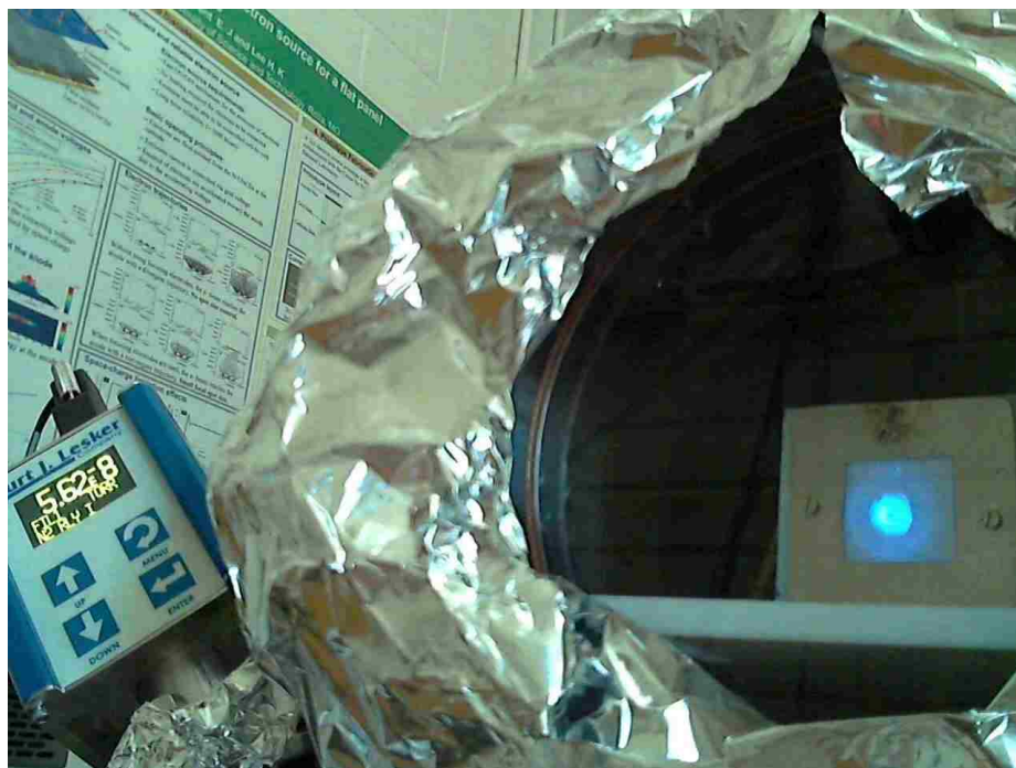
Figure 4.15. Electron beam visualization via YAG coated glass.
