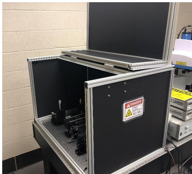
Figure 2.1: Light-proof enclosure for optical components.
