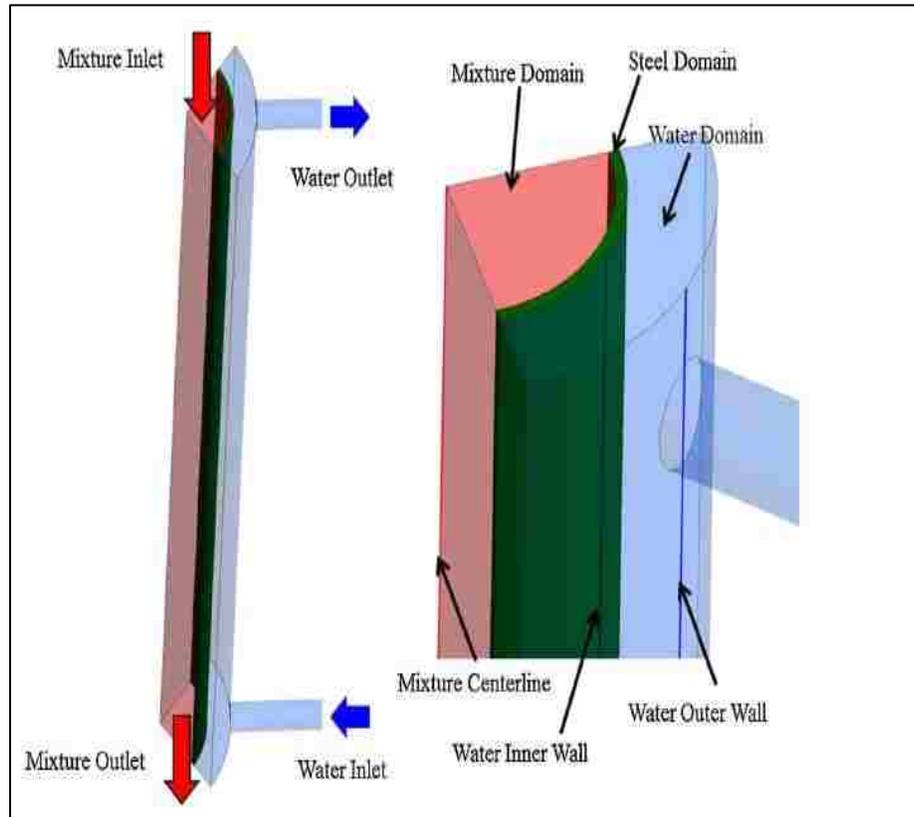
Figure 2.6 Three-dimensional model of geometry used for simulations [24]
