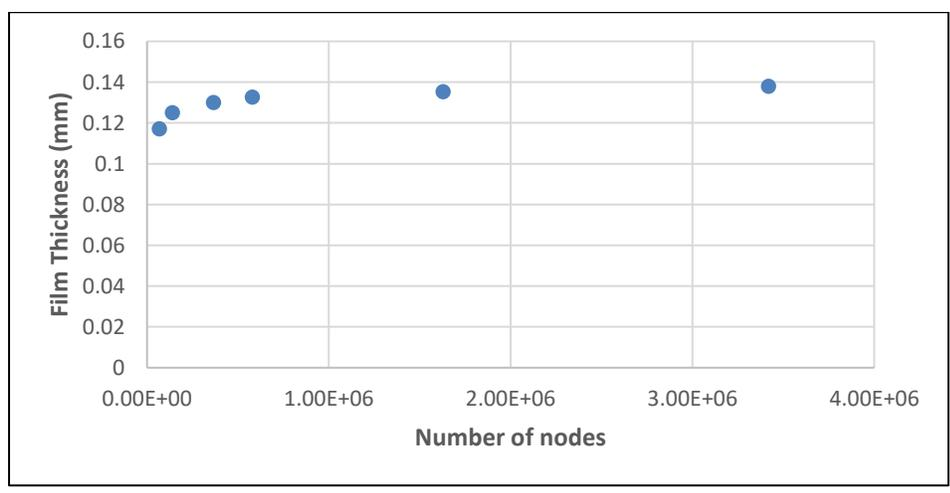
Figure 5.5 Condensate film thickness vs number of nodes
