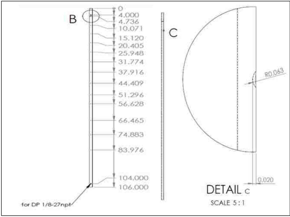
Figure 3.4 Thermistor locations on the condenser tube
