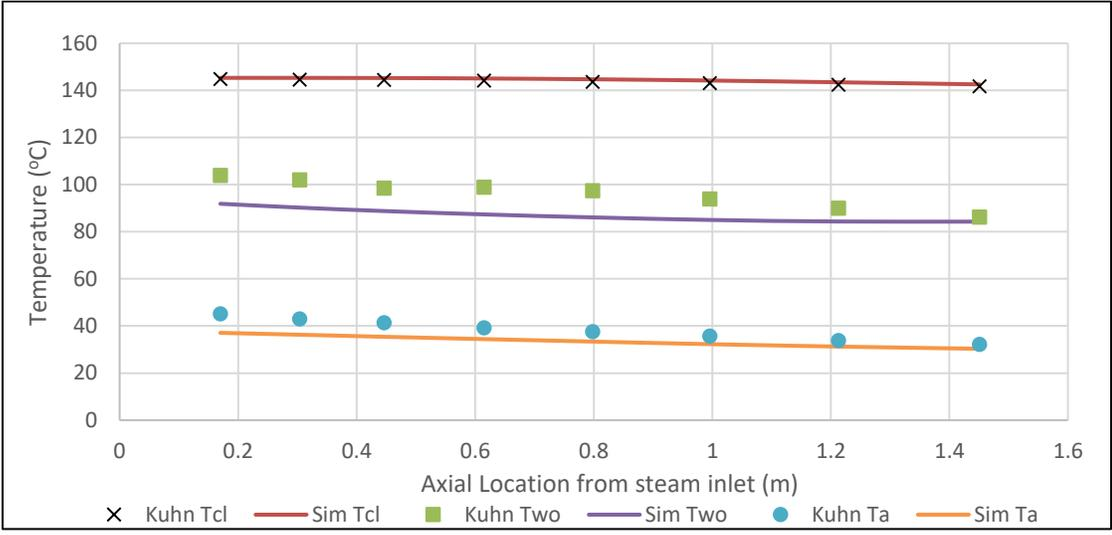
Figure 5.14 CFD results vs simulation results for Geometry 2
