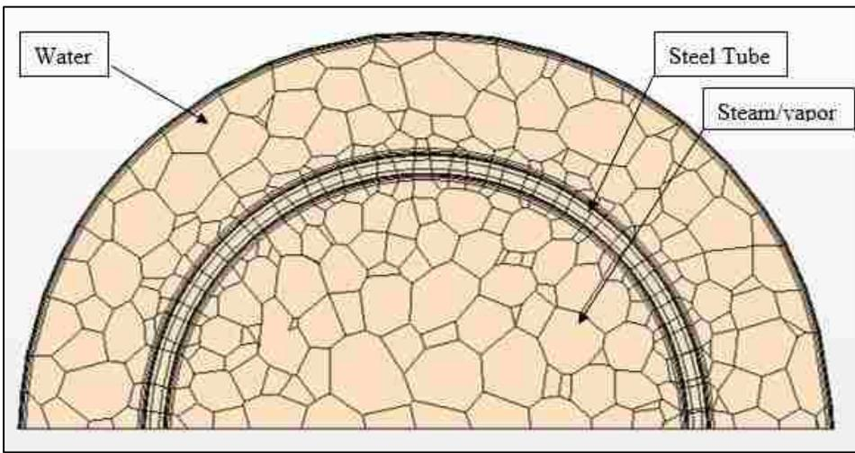
Figure 5.4 Cross sectional view of a characteristic mesh
