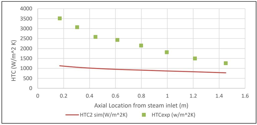
Figure 5.15 HTC comparison between CFD and experiment
