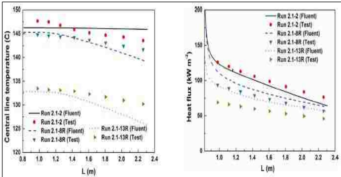
Figure 2.9 Simulation vs experimental results for steam-air mixture [25]
