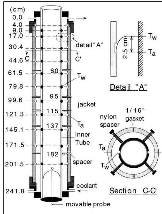
Figure 2.2 Test Section sketch of Kuhn et al. [17]
