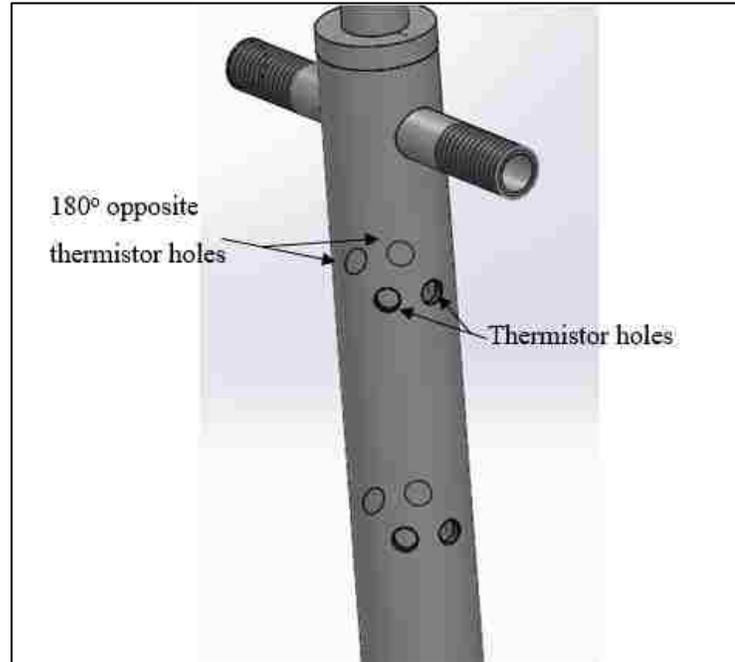
Figure 3.3 Drilled holes for thermistor placement
