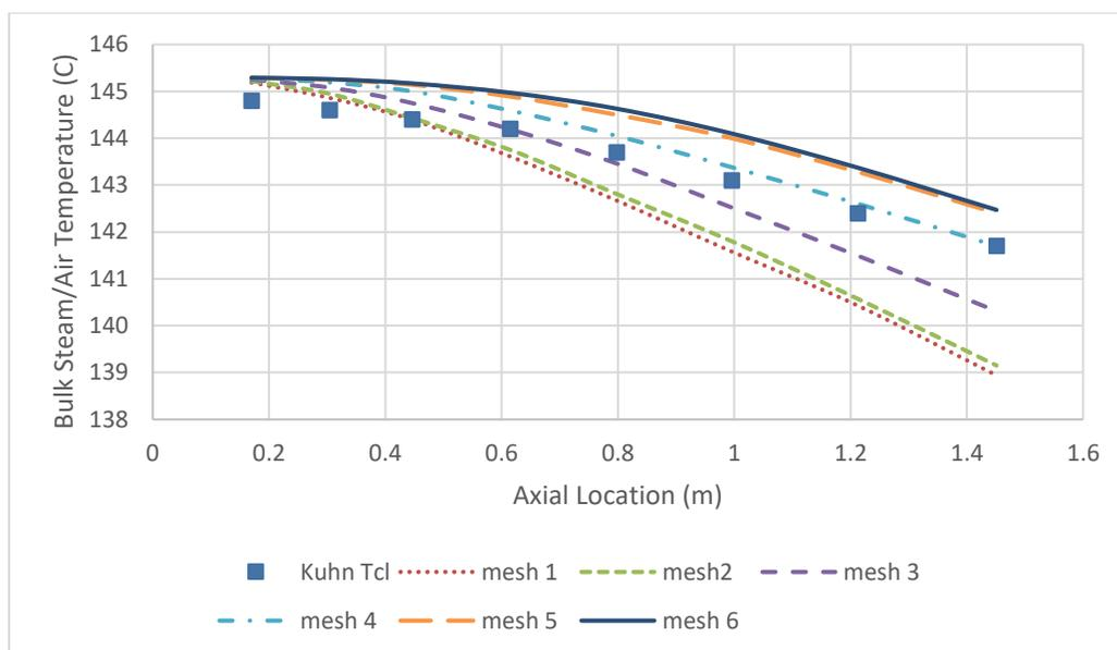
Figure 5.6 Bulk temperature distribution for different mesh sizes
