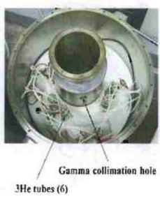
Photo of AEFC 3He Tubes and Ion Chamber
