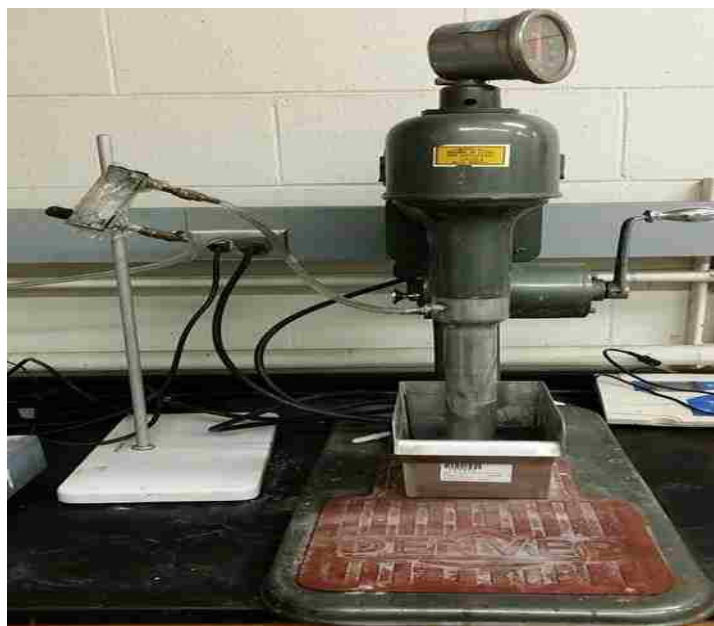
Figure 3.4. Picture of the Denver cell used in the bench-scale flotation experiments.
