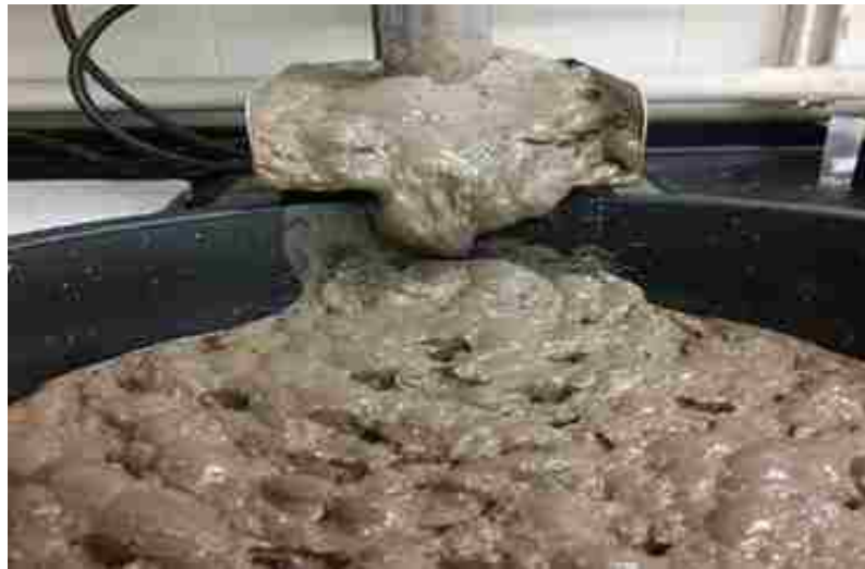
Figure 4.22. A picture of froth products collected at longer residence time (0 to 10 min) when Hy-PAM was used as a quartz depressant.
