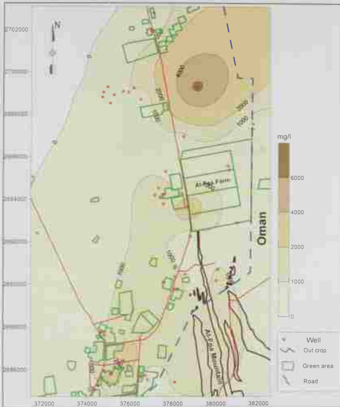
Figure (4.6) Map showing the distribution of the chloride anion (mg/l) in Al-Foah area.
