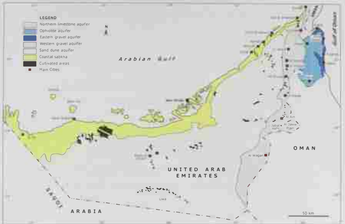
Figure (3.7) The main water bearing units (aquifers) in the United Arab Emirates (after Rizk et al, 1997 and Al-Nuaimi, 2003)
