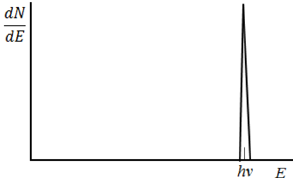
Figure 1.4. Single Peak at a Total Electron Energy Corresponding to the Energy of the Incident X-rays
