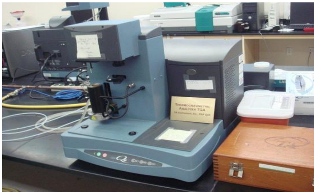
Figure 3.4. Q50 Thermogravimetric Analyzer (TGA)
