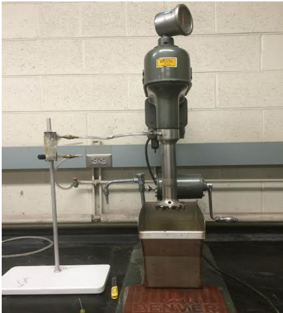
Figure 3.8. D12- Denver Flotation laboratory cell.
