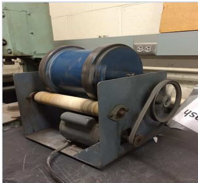
Figure 3.3. Laboratory ball mill
