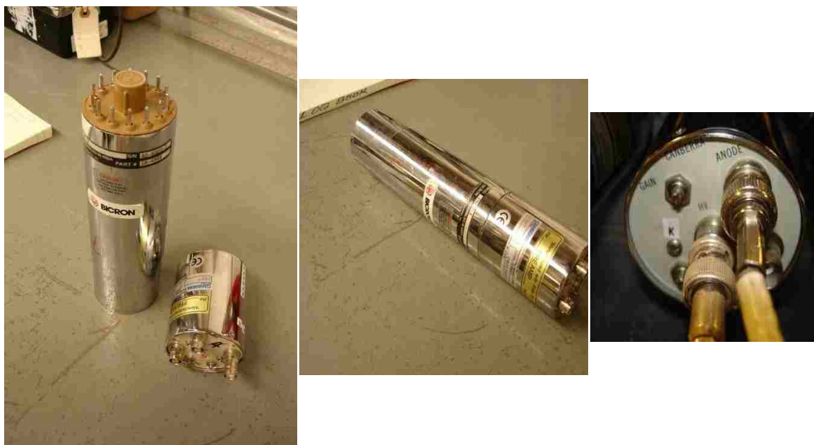
Figure 3.16: The NaI(Tl) solid state scintillation detector assembly
