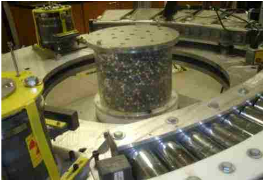
Figure 4.1: Experimental setup of a 1 ft diameter pebble bed packed with 0.5 inch glass spheres inside the CT scanner
