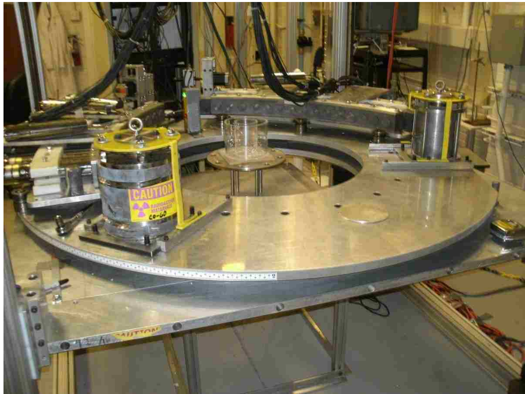
Figure 3.1: The gamma-ray DSCT measurement system
