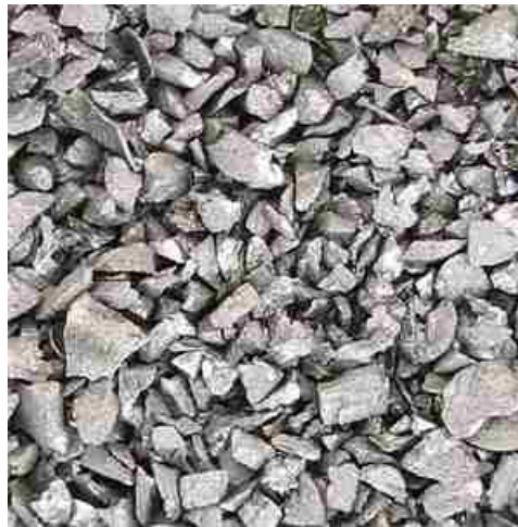
Figure 4.5 2-mm steel grit
