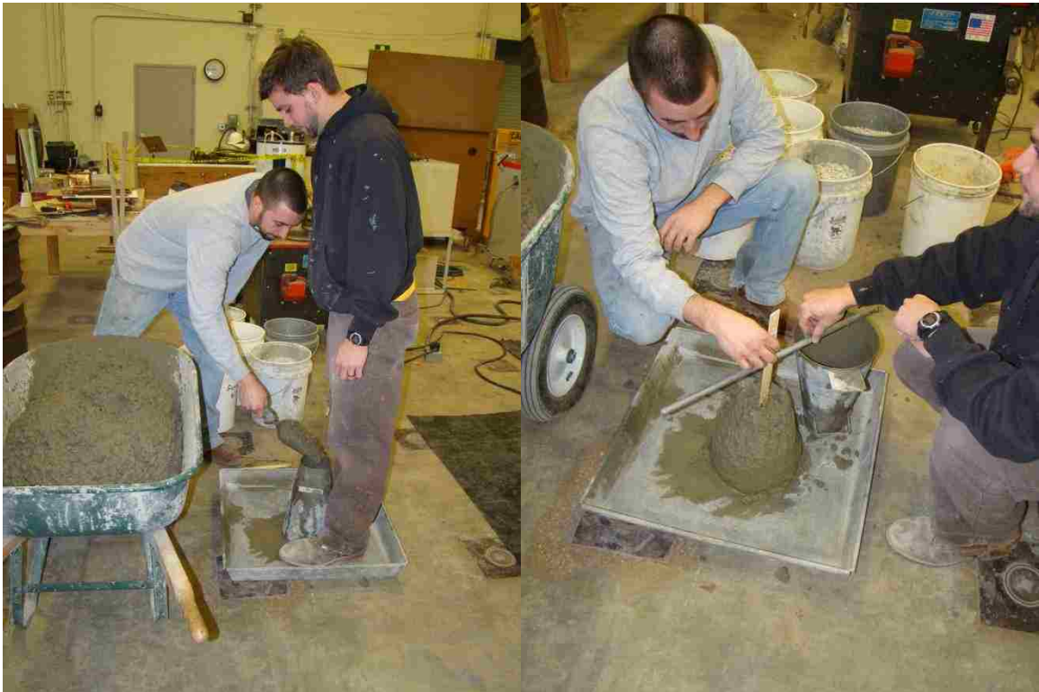
Figure 3.1 Slump test on concrete
