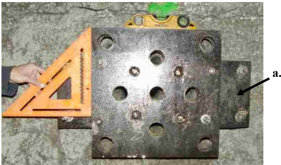
Figure 3.7. Burn Cut Drilling Template (a. Side plate extension for mounting to rock face)
