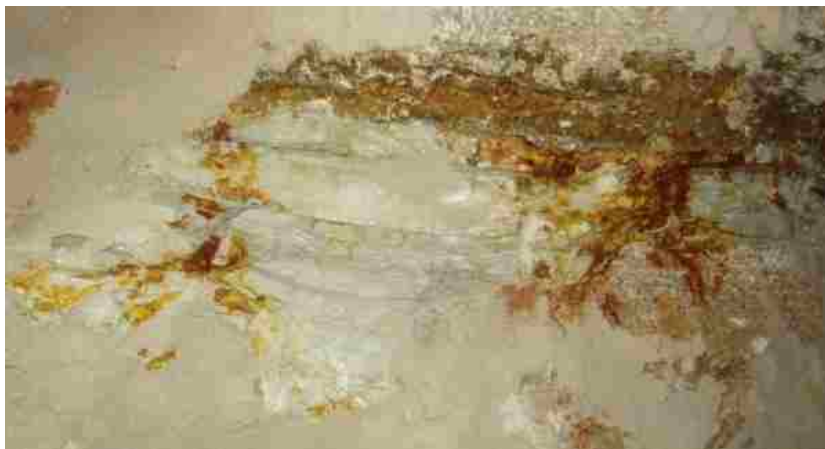
Figure 3.2. Clay and Pyrite Zone (Example of irregular rock areas located in this section of the Mine)
