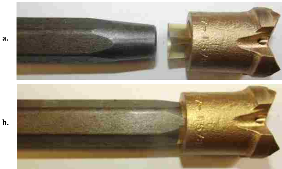
Figure 3.6. 1\frac{5}{8} inch Cross Bit and Steel (a. Unassembled and b. Assembled)
