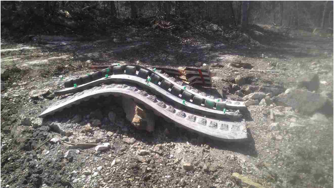
Figure 4.7 Tractor Tread Mat After Blasting
