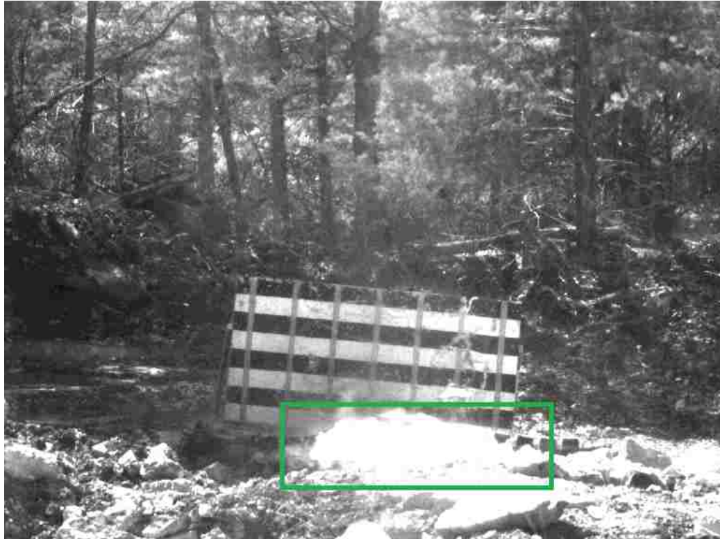
Figure 6.3 Gasses Exiting Blasting Mat after 5ms of Expansion During Test 3
