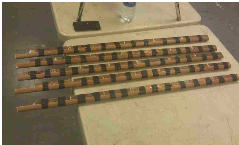
Figure 4.3 Composite Linear Shaped Charge, Constructed of Surplus End Pieces
