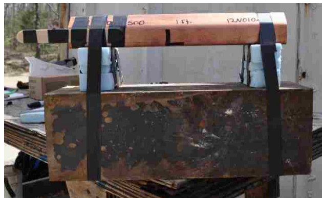
Figure 4-6. 10,500gr/ft. LSC and target with one charge diameter standoff
