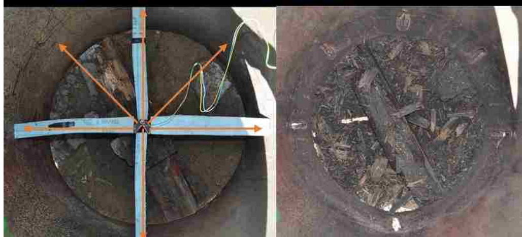
Figure 5-3. Pipe test before (left) and pipe test (after) charge detonation. The impact profile on the pipe shows the liner was directly projected off of the faces of the LSC.
