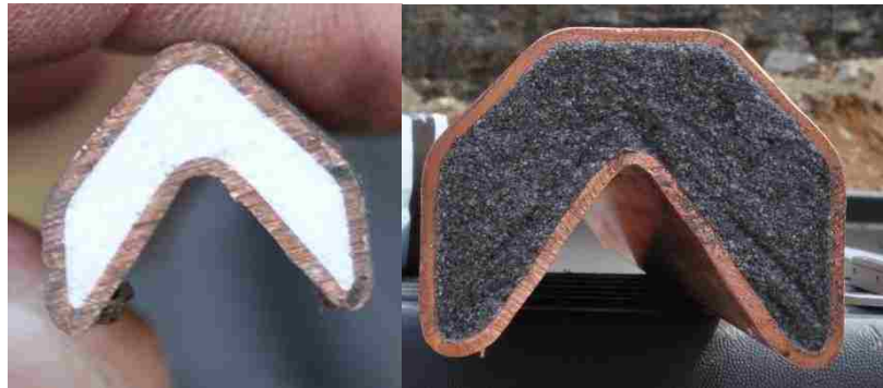
Figure 2-4. Typical LSC (left) 10,500 gr/ft. LSC (right).
