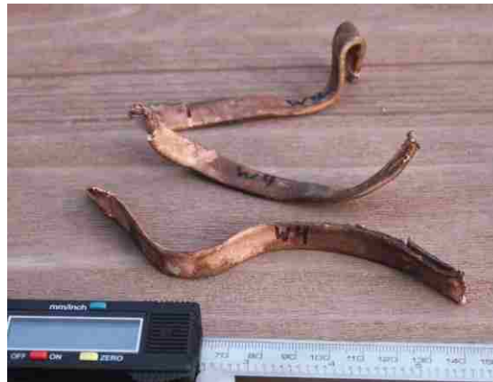
Figure 2-7. Recovered LSC blade segments using a water catch system (Tabacchi, 2014).
