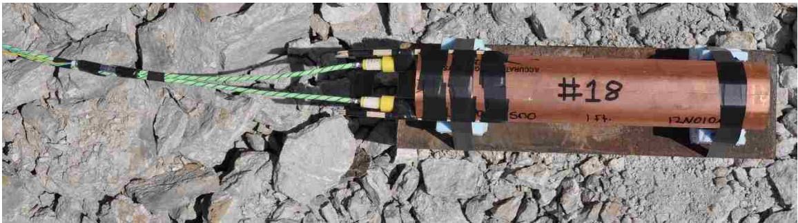
Figure 4-5. Final charge setup. When the initiation system was attached to the charge it was important to ensure the length of explosives from the cap to the LSC was kept the constant. This would ensure a simultaneous initiation of the LSC.
