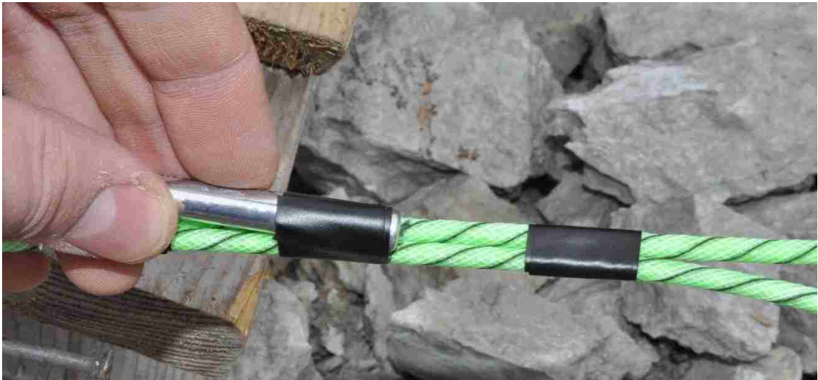
Figure A. 8: Securely attach the blasting cap so that it is in line with the measured marks
