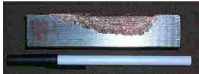
Figure 3-5. Observed cut profile of single end initiation (pen for scale) (Lim, 2003). The cut profile observed in this target block is a fairly representative cut profile. The zones of run-up, cut and run-down are clearly visible. This initiation method performed as hoped and is recommended by Lim as viable initiation method that produces an acceptable cut profile.
