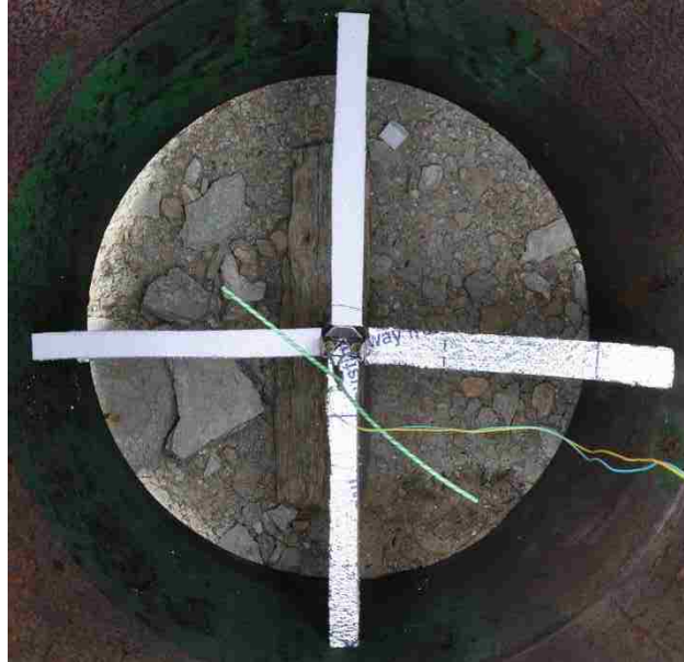
Figure 4-9. Charge position inside pipe. The foam standoffs were used to keep the sides of the charge, the top of the charge and the lower tips of the charge legs equidistant from inside of the pipe. This setup was meant to ensure the LSC fragments traveled the same distance before impacting the pipe.
