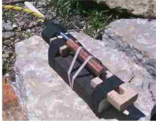
Figure 3-4. Single end initiation test setup (Lim, 2003). This initiation method places a cap at one end of a LSC aiming to start the detonation at one side of the LSC and have it progress to the other.
