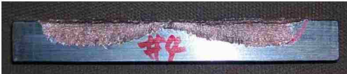
Figure 3-7. Midpoint initiation cut profile. This cut profile show that the midpoint initiation method did not increase the cut performance of the LSC instead it nearly doubled the zone of run up.
