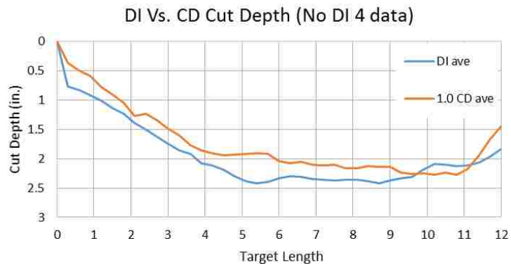
Figure 5-2. Comparison of cut depth DI tests vs. 1.0 CD tests (no DI 4 data). Note, the curve that initially tracks lower is the plot for the DI data (a difference between the curves' colors may only be apparent in color copies of this document).
