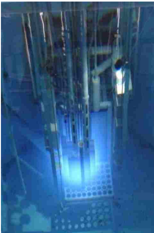
Figure 5.1. Picture of MSTR working at full power (200kW).
