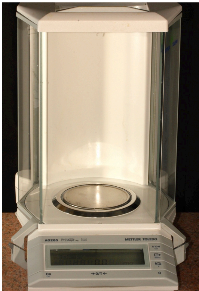
FIGURE 7. Digital analytical balance (Mettler Toledo, Columbus, OH).
