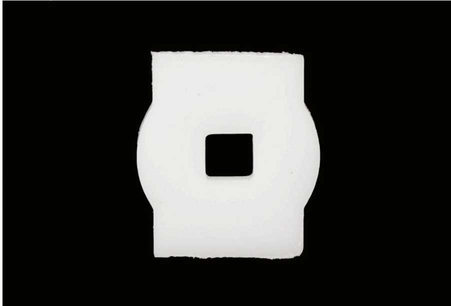
FIGURE 4. A square customized Delrin plastic mold 5 \times 5 \times 2 mm.
