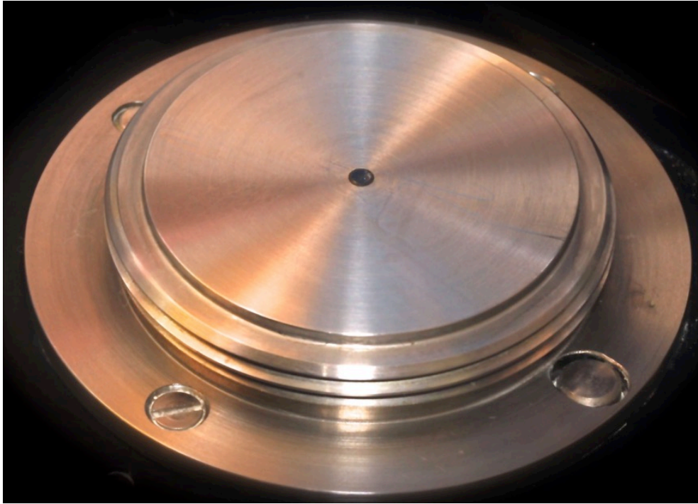
FIGURE 14. The ATR-FTIR diamond was cleaned with an ethanol wipe.
