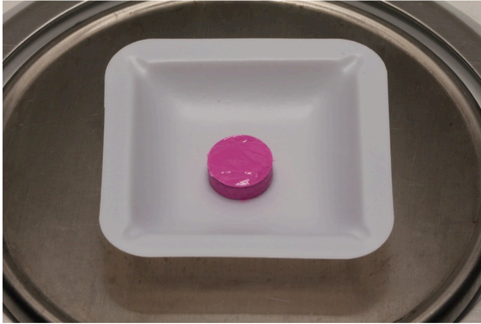
FIGURE 11. The tested specimen and the impression material (Impression + specimen) were weighed together (SP) to determine the pre-application weight of the impression material (P1).
