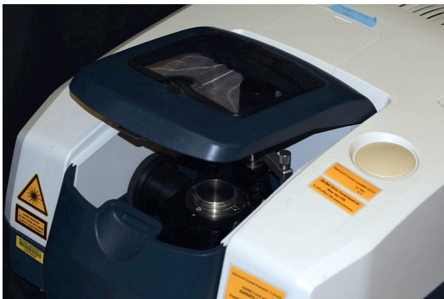
FIGURE 13. The Fourier transform infrared spectrophotometer with a diamond attenuated total reflectance attachment (FTIR-ATR).
