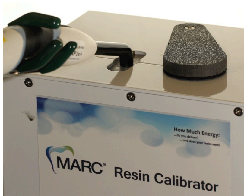
FIGURE 3. LCU tip was aligned with the MARC-RC crosshead on the surface positioned flat and perpendicular against the sensor to standardize the x-, y-, and z-directions.
