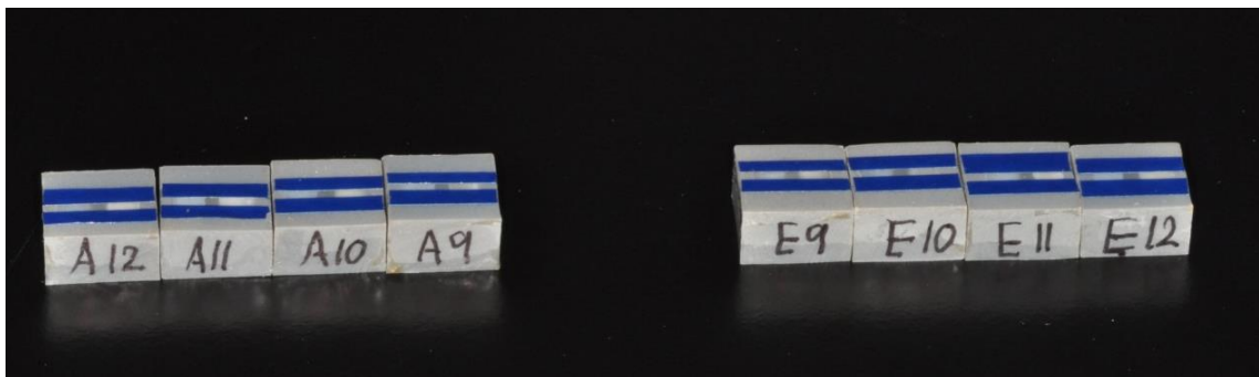
FIGURE 10. Specimens' reference surfaces covered with UPVC tape.
