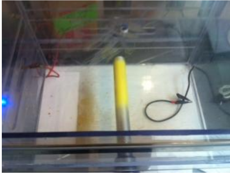
FIGURE 9. Electrospinning of scaffold on mandrel during process.
