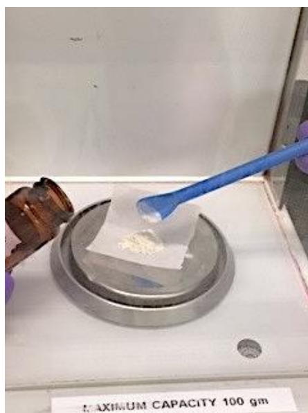
FIGURE 2. Dried HNT-encapsulated with CHX powder weighed and incorporated into the adhesive.
