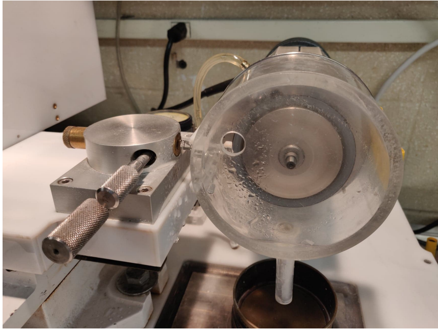
FIGURE 9. A figure shows the sectioning of the specimen by Series 1000 Deluxe' hard tissue microtome.
