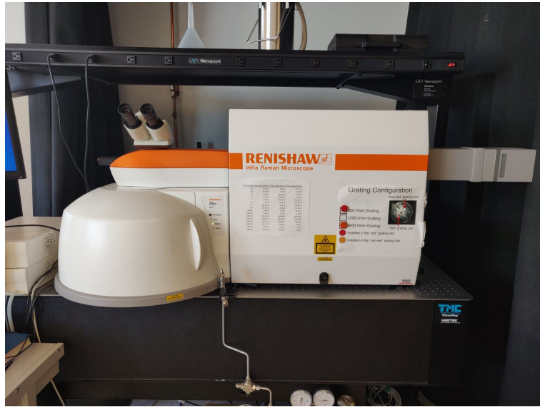
FIGURE 11. A figure shows Spontaneous Raman spectroscopy (SpRS) in Via Renishaw microscope.
