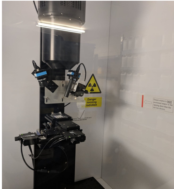
FIGURE 10. A figure shows X-ray instrument (VHR X-Ray, USB Camera DFK 42BUC03 with Tamron Lens).
