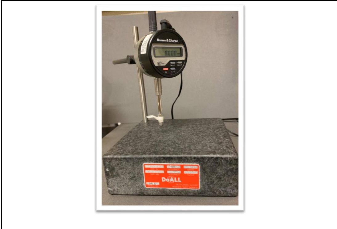
FIGURE 2. Micrometer used for measurement during grinding.
