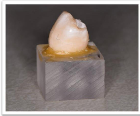
FIGURE 1. Sectioned premolar at CEJ fixed on acrylic block with cyanoacrylate adhesive and sticky wax.
