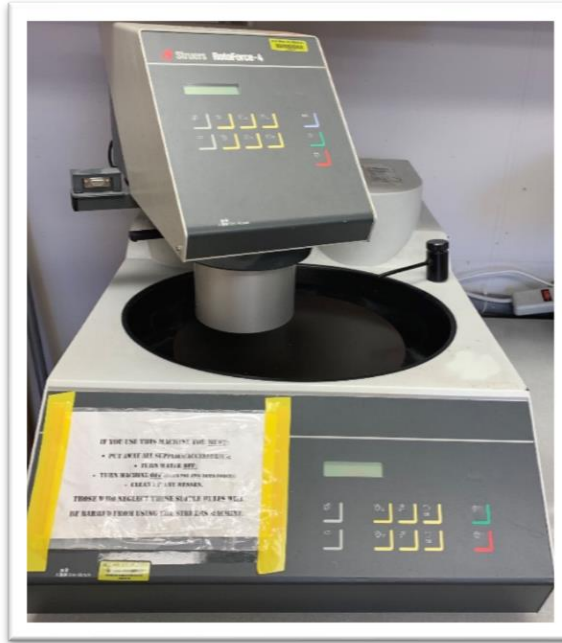
FIGURE 3. Struers machine used for grinding by diamond abrasive discs.
