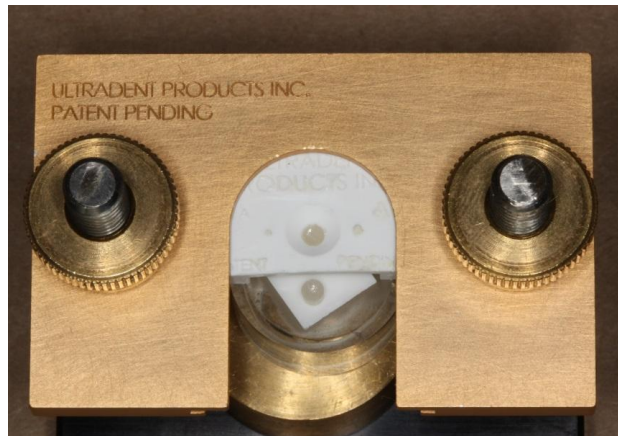
FIGURE 7. Bonding of Zirconia sample with Ultradent Jig.
