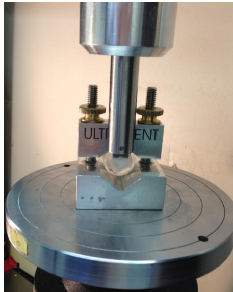
FIGURE 14. Illustration of sample going for shear bond strength test in universal testing machine
