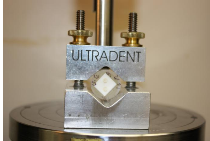
FIGURE 13. Illustration of samples arranged in Ultradent jig for shear bond strength testing.
