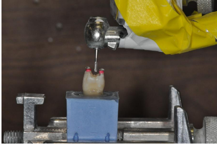
FIGURE 4. The mounted teeth and a high-speed contra angle air-turbine handpiece were positioned on an A.M.D. surveyor.
