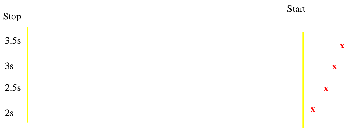
Figure 20: Start time tests for trajectory Method Conducted with Alumina paste at Times of 3.5 s, 3.0 s, 2.5 s and 2.0 s. Standoff Distance is 55%. Extrusion Force is 450 N. Table Velocity is 4.9 mm/s. ‘x’ Controller On.
