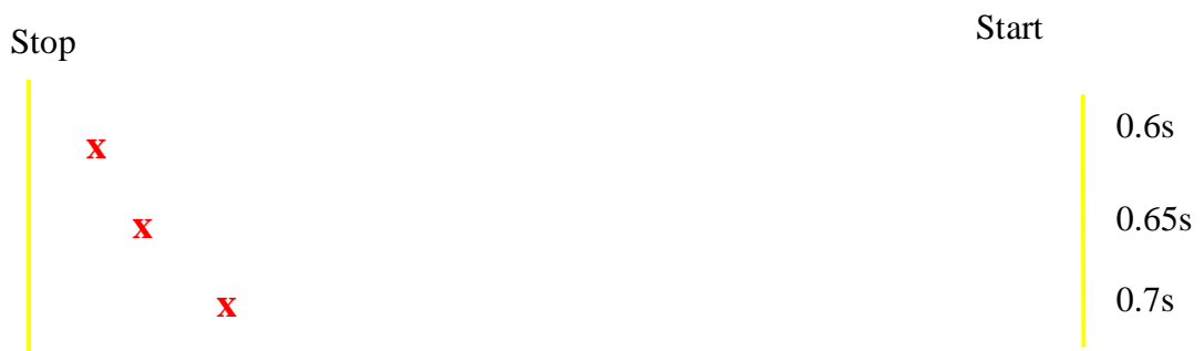
Figure 21: Stop Time Tests for Trajectory Method Conducted with Alumina Paste at Times of 0.7 s, 0.65 s and 0.6 s. Extrusion Force is 450 N. Table Velocity is 4.9 mm/s. Standoff Distance is 55% of Extrudate Diameter. ‘x’ Controller Off.
