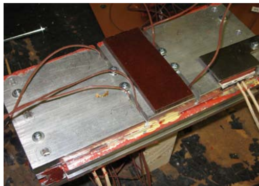
Figure 3.15: Phenolic piece positioned on heater
