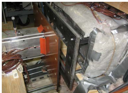
Figure 3.34: Aligning test section with outlet settling chamber flange
