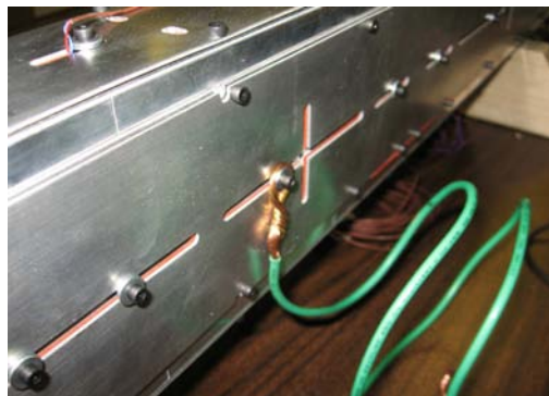
Figure 3.28: Ground wire attached to test section
