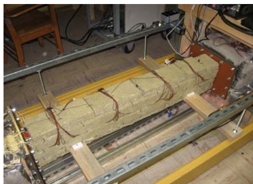
Figure 3.37: Mineral wool insulation on test section
