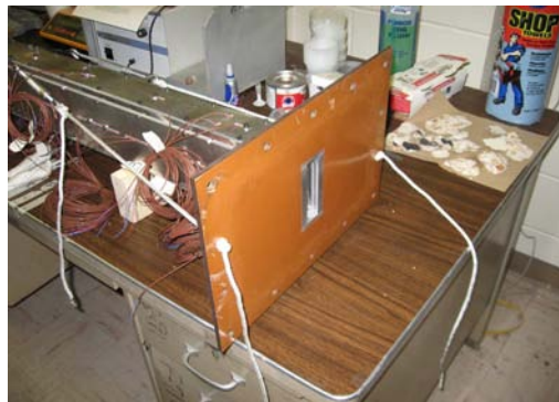
Figure 3.30: Knots tied outside of phenolic flange
