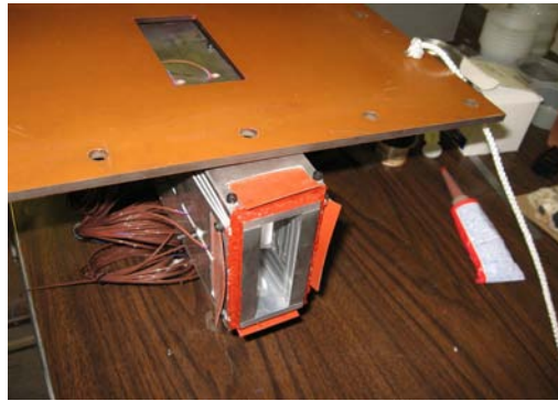
Figure 3.32: RTV silicone applied to test section
