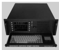
Figure 2.2. Rack Mountable Speedgoat Target PC.
