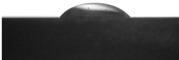
Figure 7. Image of film droplet used for interferometric film thickness measurement validation.
