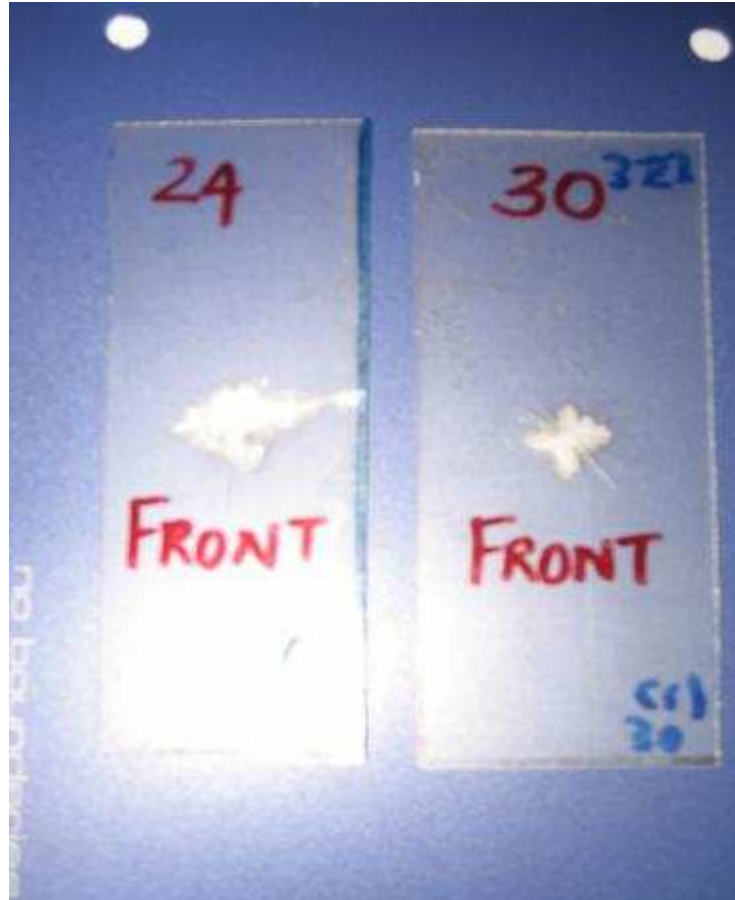
Figure 5.19: Front View of the Damage Caused by Impact Testing
