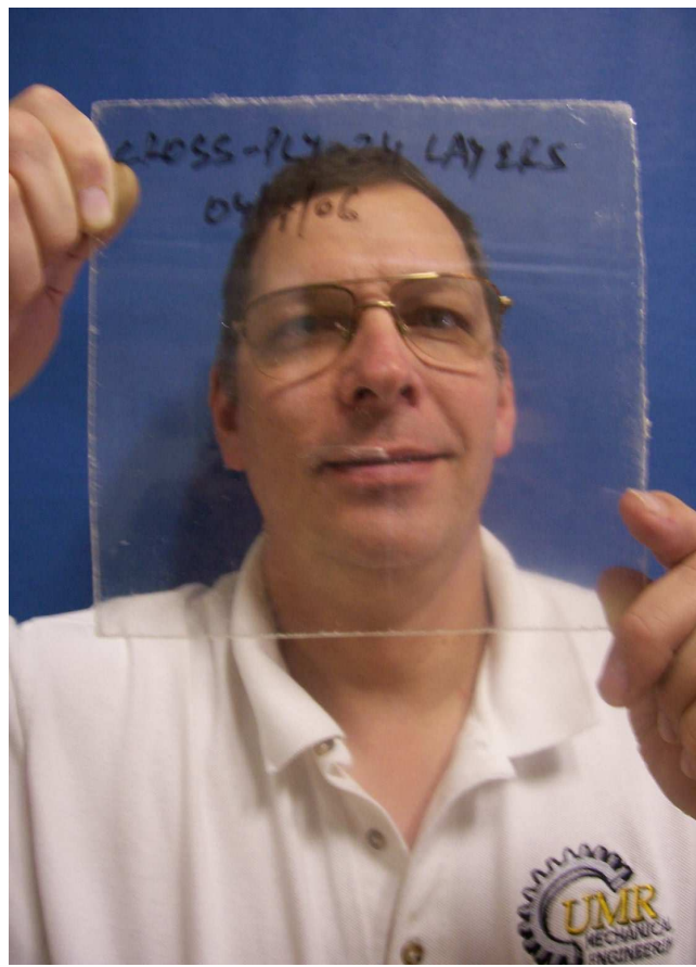
Figure 4.3: Glass Ribbon Reinforced Transparent Panel Manufactured at UMR
