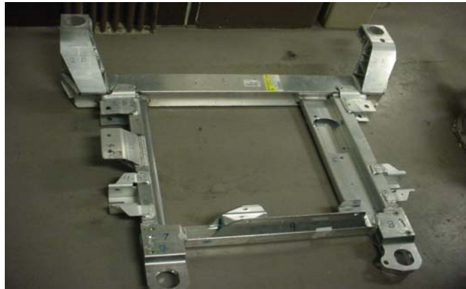
Figure 16: Aluminum Chassis Used for Performance Feasibility Study
