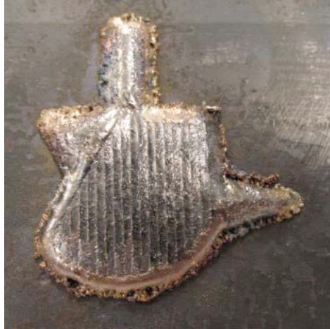
Figure 2.4: Hybrid Tool Path Part Built by Computer Control
