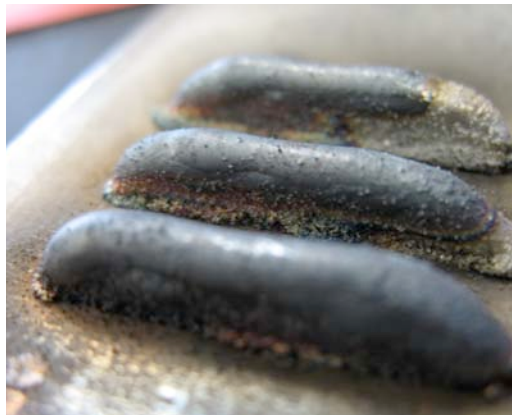
Figure 2.3: Thin Walls Built by Computer Control
