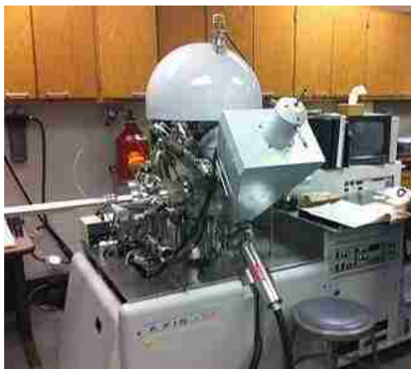
Figure 4.7. Left side: KRATOS AXIS 165 X-ray Photoelectron Spectrometer (XPS) located at the materials research center (MRC) on campus.
