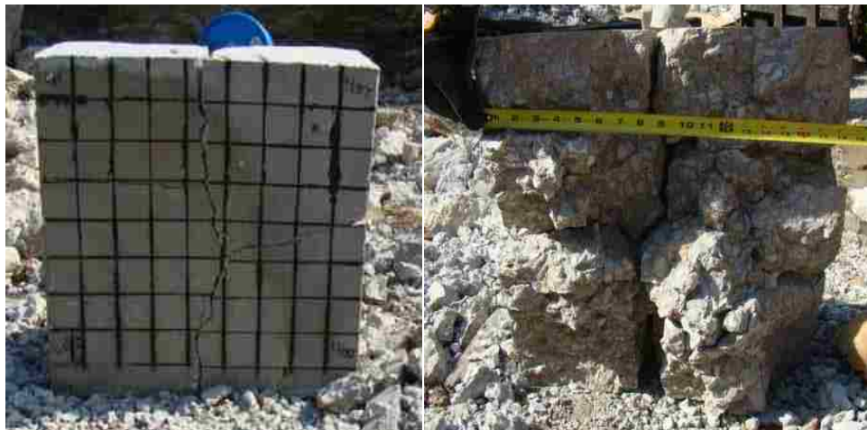
Figure 4.7: Block 4, back face and interior views, after impact.
