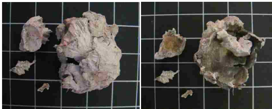
Figure 4.26: Recovered pieces of Projectile 23
