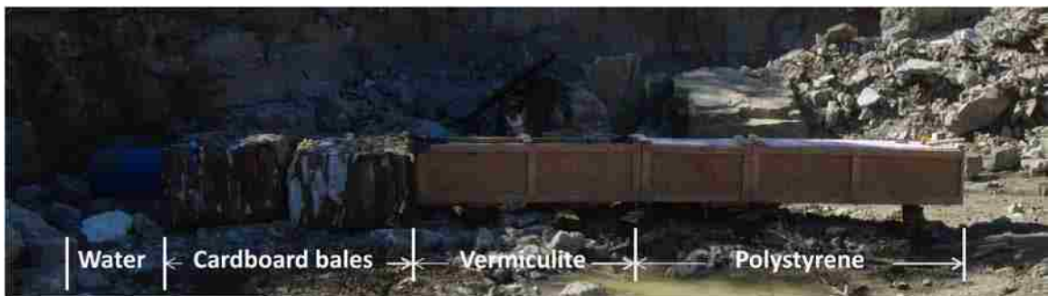
Figure 3.5: Soft recovery system.
