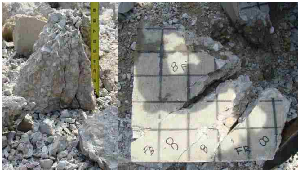
Figure 4.13: Block 8, center and recovered front pieces after impact.
