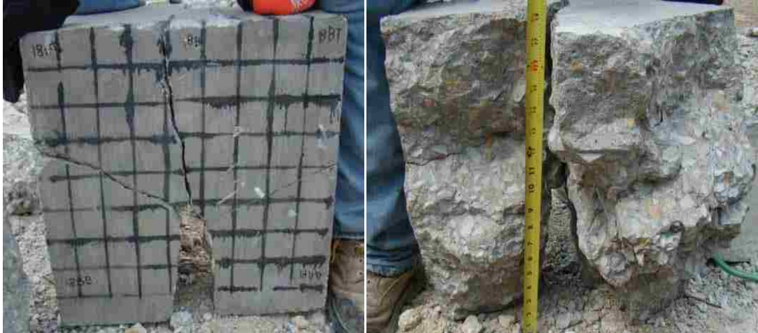
Figure 4.23: Block 18, back face and interior views after impact
