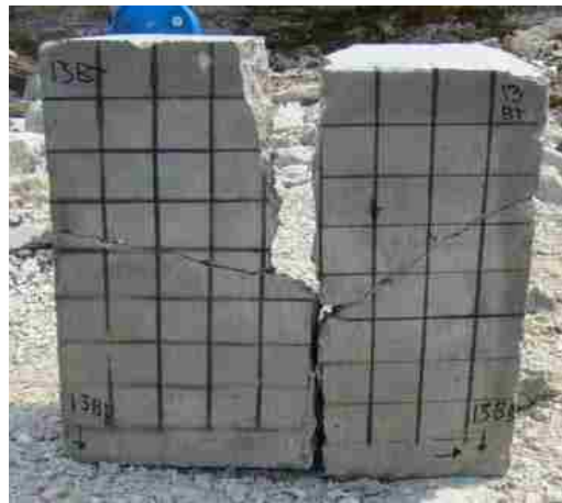
Figure 4.18: Block 13, back face after impact
