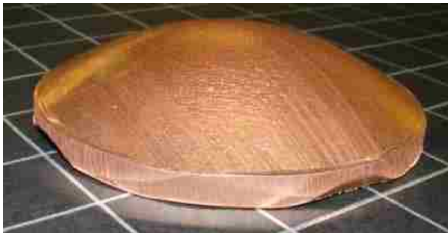
Figure 3.1: Completed flyer plate.
