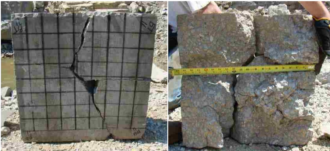
Figure 4.16: Block 11, back face and interior views after impact
