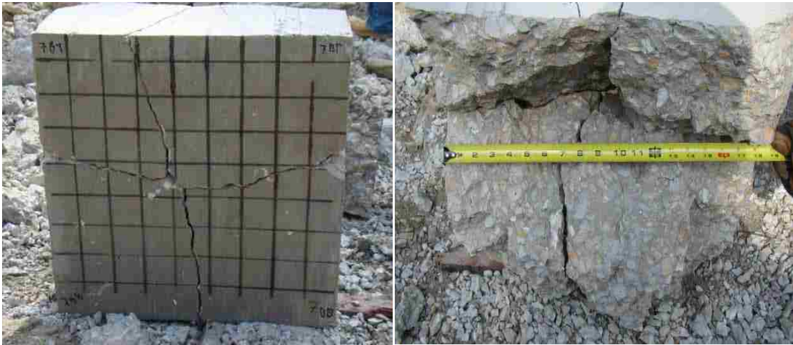
Figure 4.10: Block 7, back face and interior views after impact.
