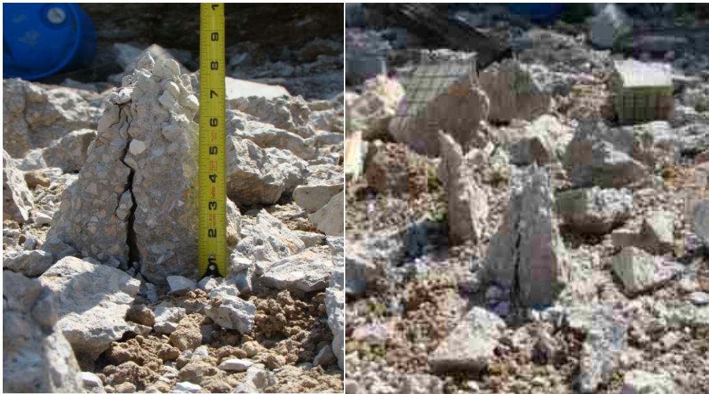
Figure 4.5: Block 2, concrete scatter after impact.
