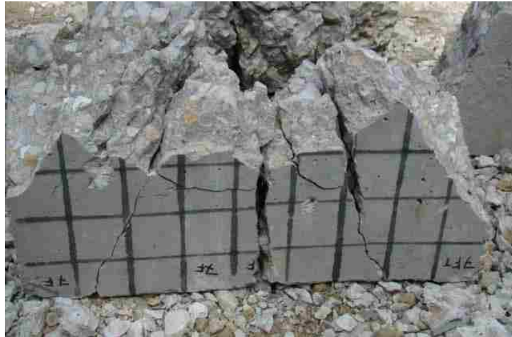
Figure 4.11: Block 7, front face pieces recovered after impact.
