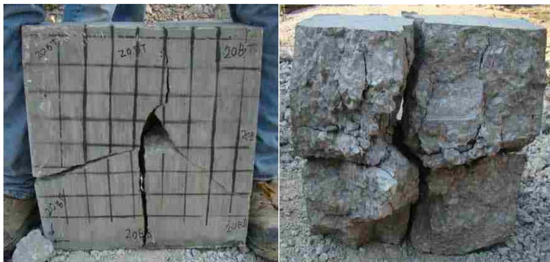
Figure 4.25: Block 20, back face and interior views after impact
