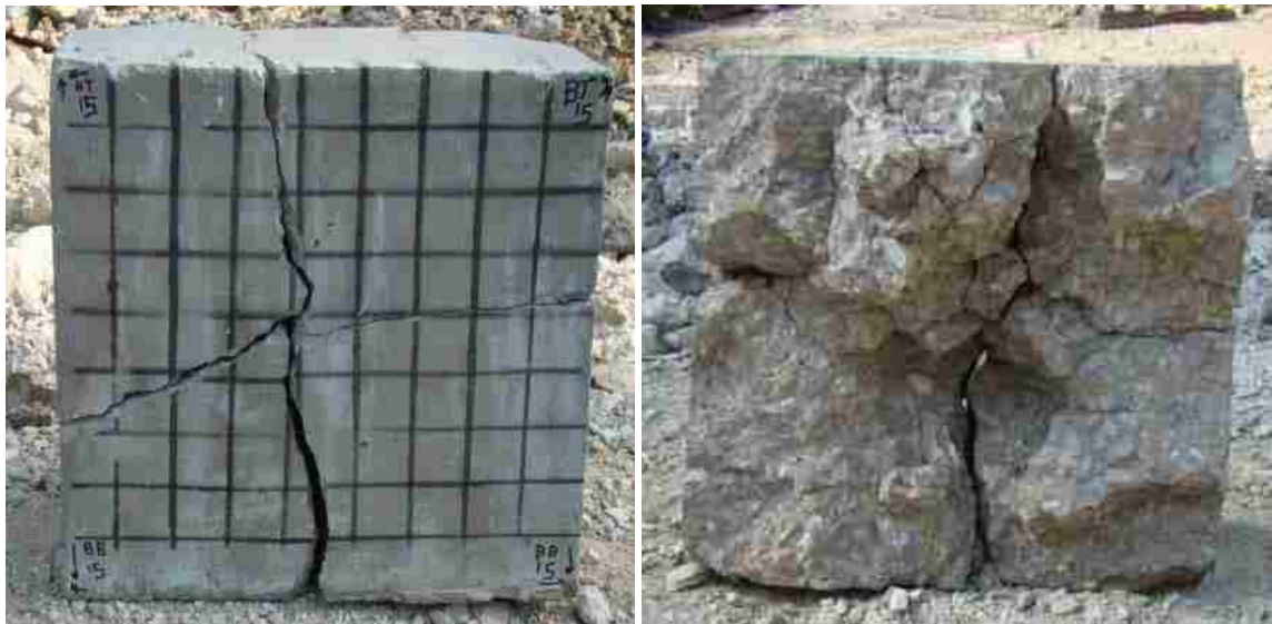
Figure 4.20: Block 15, back face and interior views after impact
