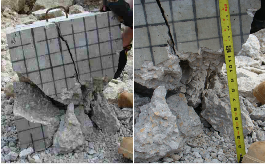
Figure 4.14: Block 9, front face after impact.
