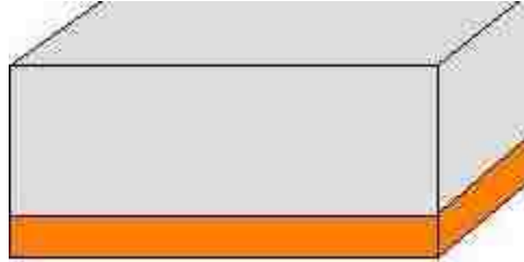
Figure 4.8 Open-Faced-Sandwich Gurney Equation Configuration
