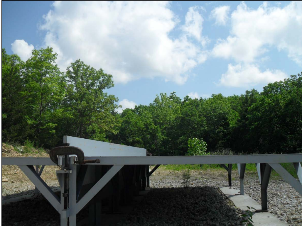
Figure 3.7. Blast table with wall height of 226 mm.
