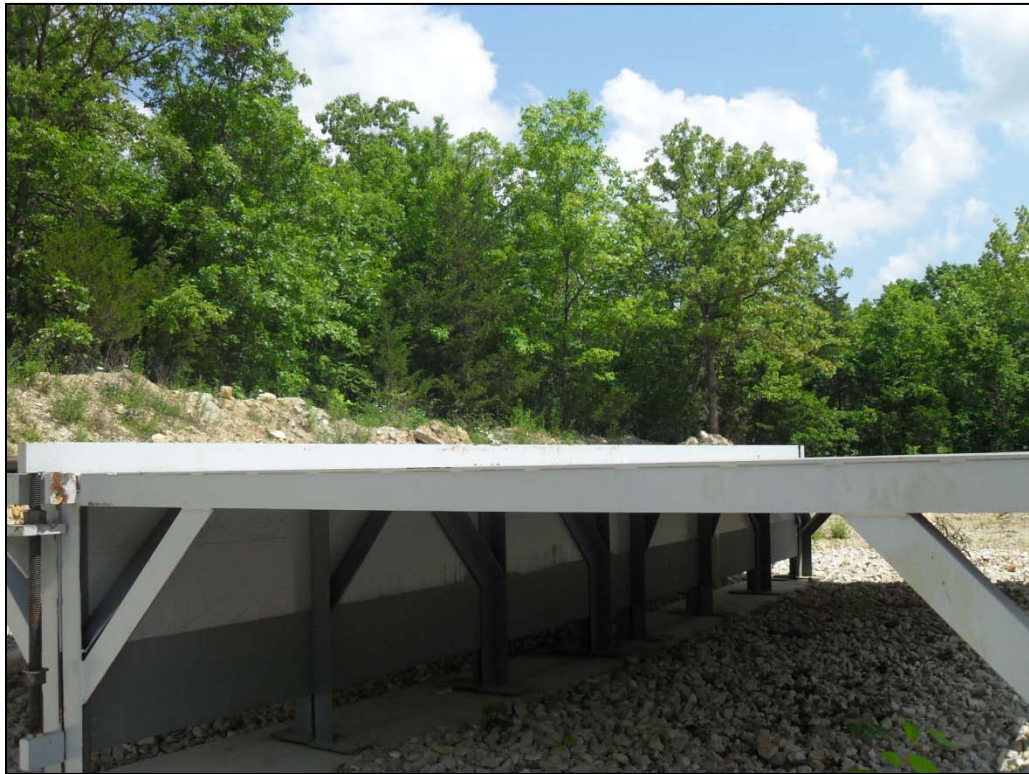
Figure 3.6. Blast table with wall height of 73 mm.
