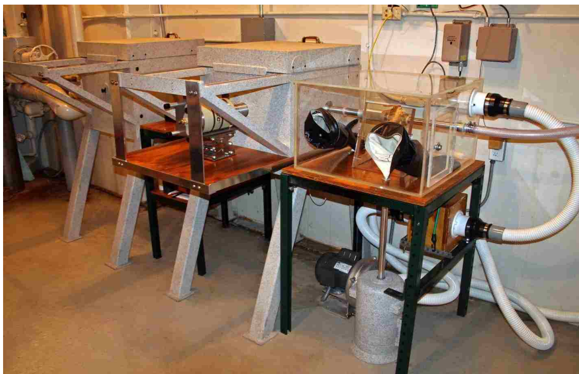
Fig. 9. Hot Cell System with HPGe Detector
