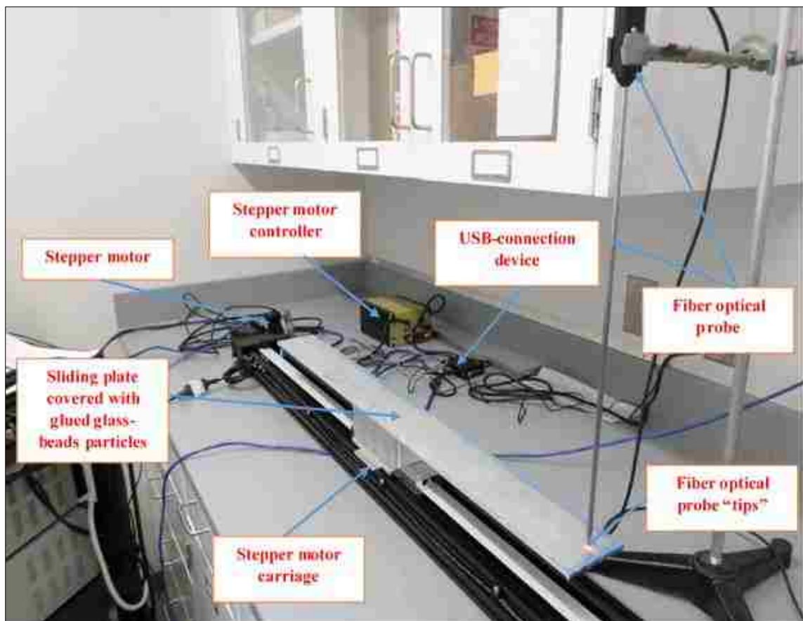
Figure A.4. Optical fiber probe and belt-driven stepper motor calibration setup for the solid particle velocity.
