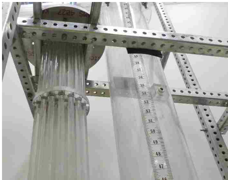
Figure 2.5. Photo of 0.0127 m vertical internals and its support.
