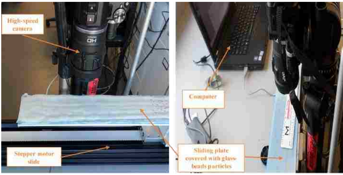
Figure A.6. A high-speed camera and belt-driven stepper motor setup for the validation of the solids particle velocity.
