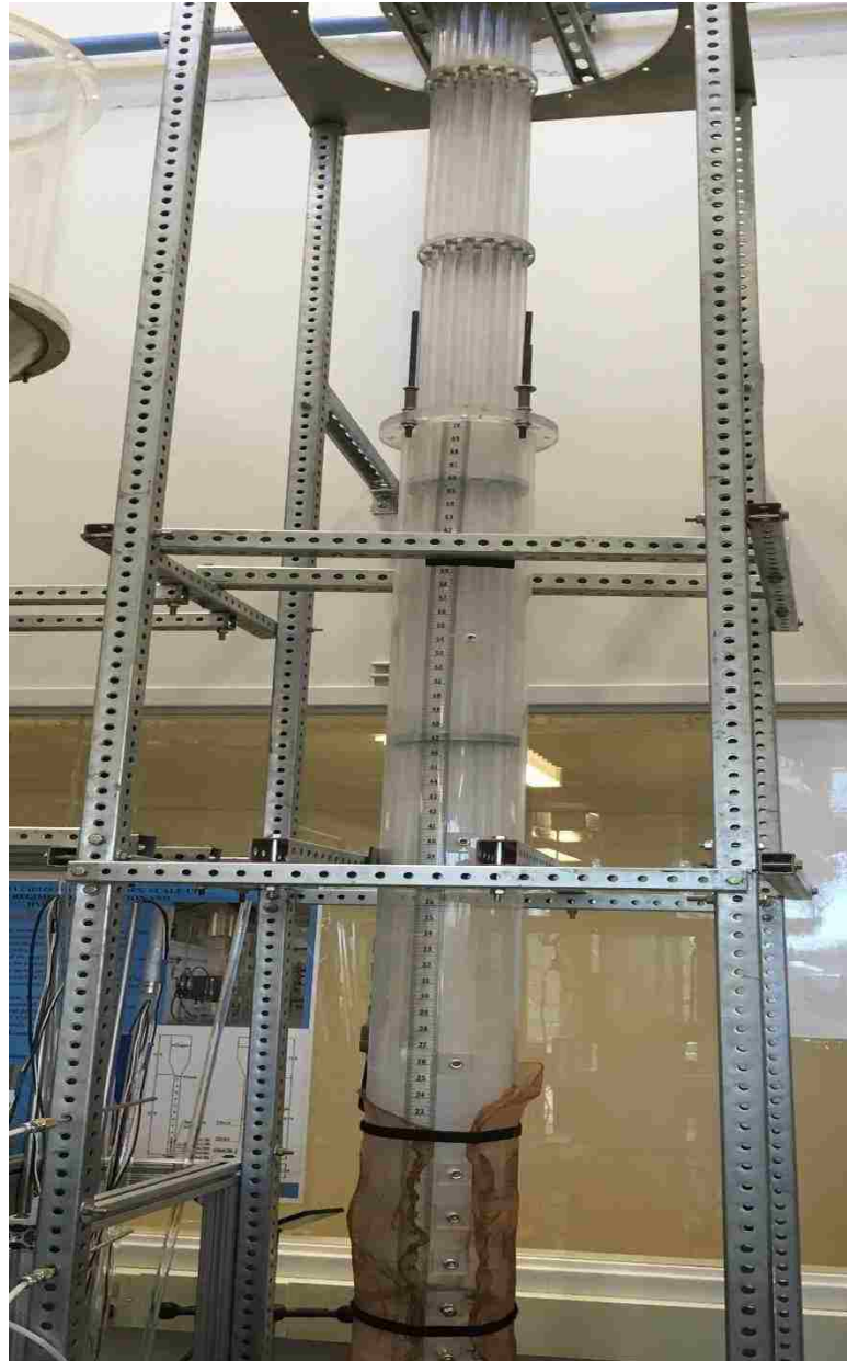
Figure 2.2. Photo of the fluidized bed column with internals.
