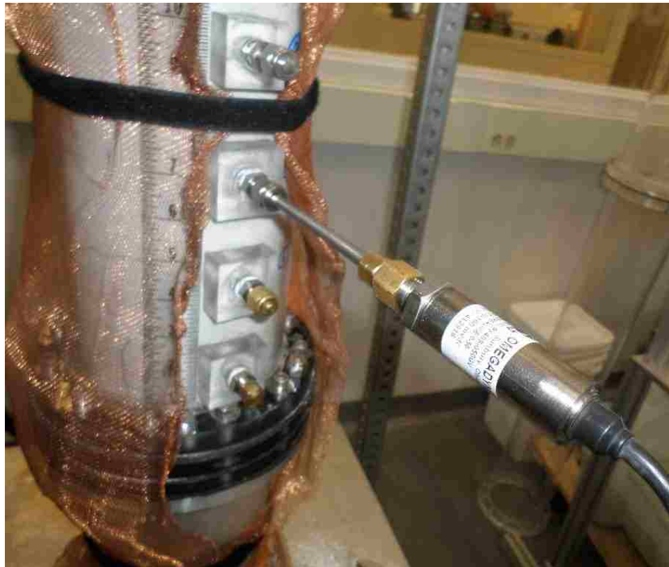
Figure 4.1. The local pressure probe connected to a single-ended pressure transducer (0.14 m inside diameter fluidized bed column).
