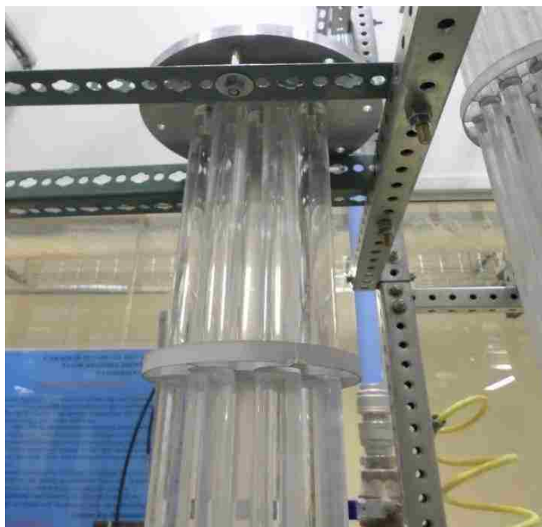
Figure 2.6. Photo of 0.0254 m vertical internals and its support.
