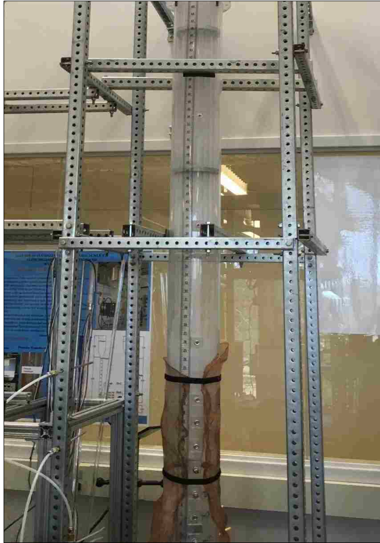
Figure B.2. Fluidized bed column with metallic structure and copper wire mesh.
