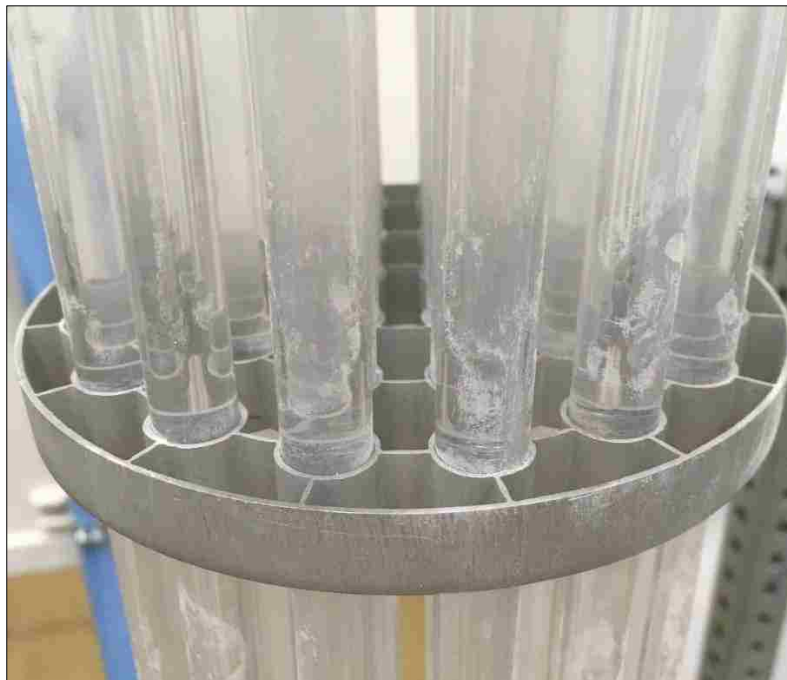
Figure 2.4. Photo of the internals configuration and its support.
