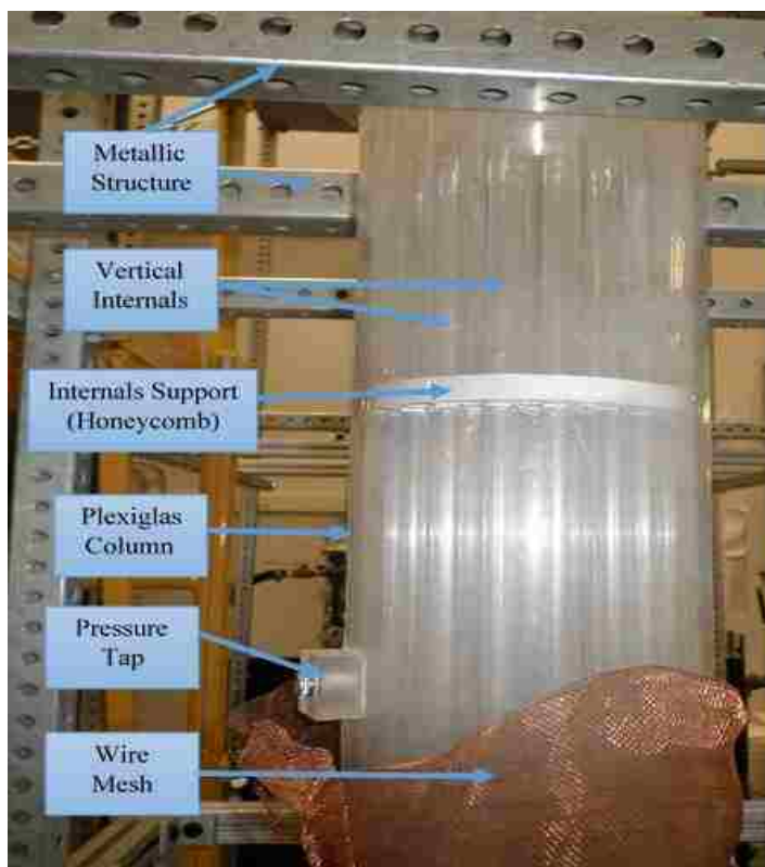
Figure 2.2. Photo for the fluidized-bed column with internals.
