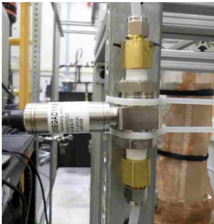
Figure 3.1. Photo of the differential pressure transducer (Omega Inc.) used in the present work.
