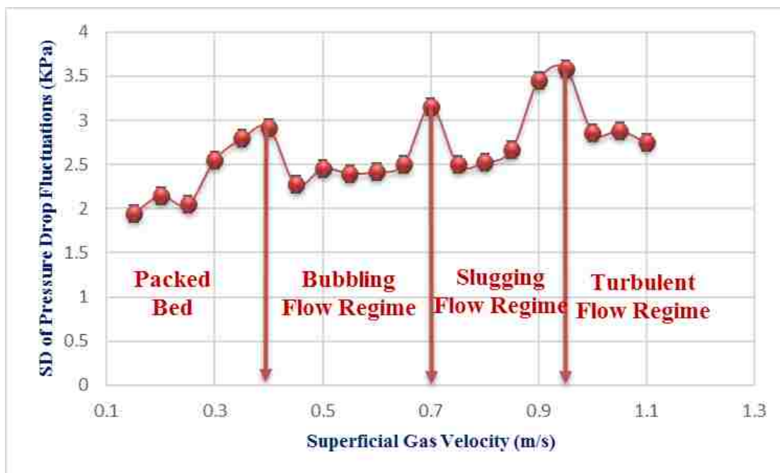
Figure 5.16. Standard deviation of pressure drop fluctuations vs. superficial gas velocity for the aluminum oxide solid particles with 0.0254 m internals.
