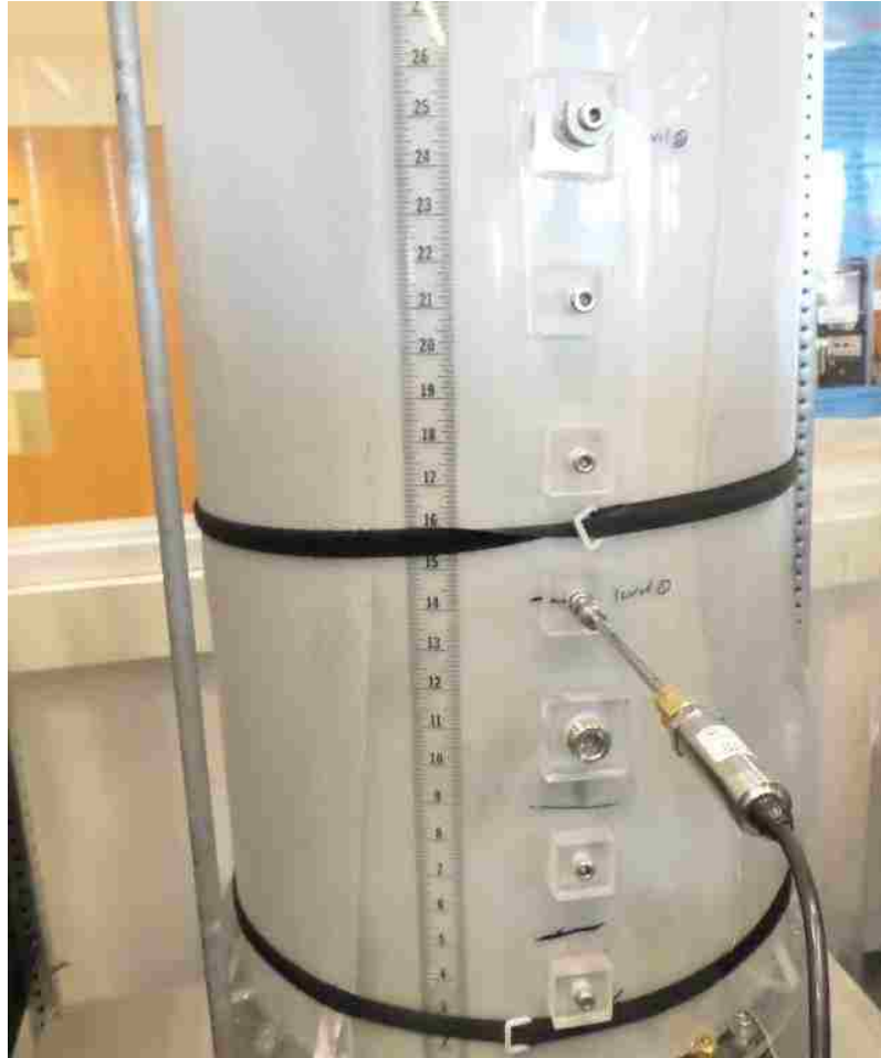
Figure 4.2. The local pressure probe connected to a single-ended pressure transducer (0.44 m inside diameter fluidized bed column).
