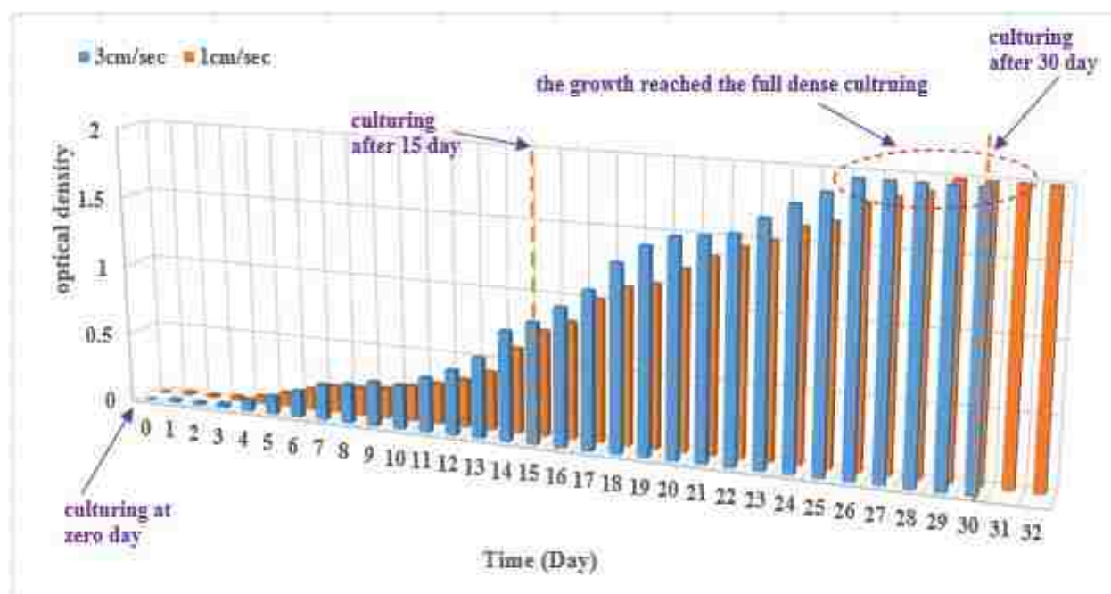
Figure 18: Optical density measurements for microalgae during the culturing system at various superficial gas velocity 3cm/s and 1 cm/s.
