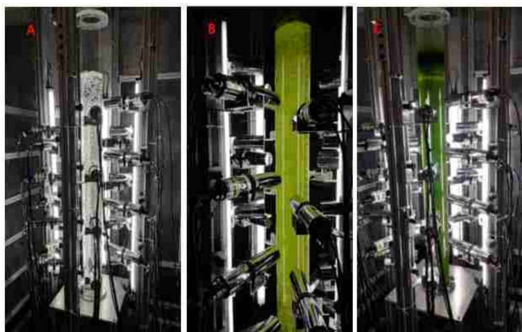
Figure 8: Microalgae culturing at different stage (A) air-water (B) air-water-15day (C) air-water-30day.
