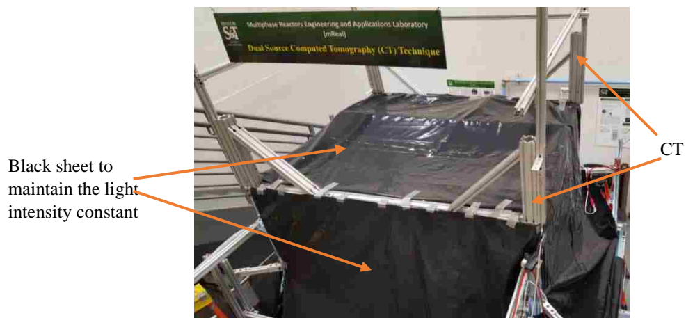
Figure 3: Black sheet was covered the CT structure in order to maintain the light intensity for photosynthesis reaction.
