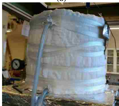
Figure 4. (a, b) Pictorial representation of the upper plenum before and after insulation
