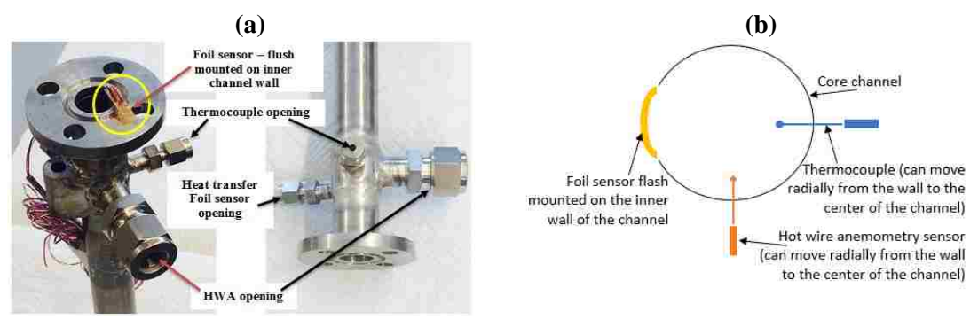
Figure 18. (a) Physical picture and (b) Schematic diagram of the novel integration of heat transfer and gas velocity measurement techniques within the connection blocks
