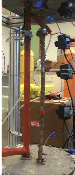
Figure 7. Electrical heaters wrapped around the heated channel
