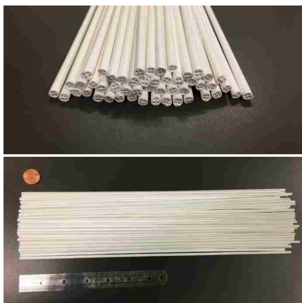
Figure 1. Photos of four-channel structured \alpha -Al 2 O 3 hollow fibers.
