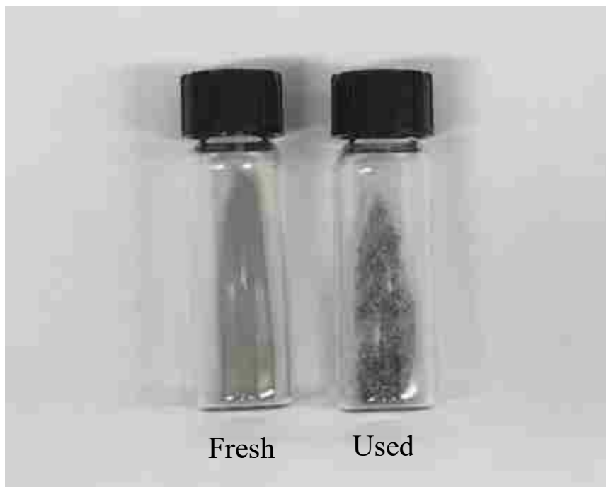
Fig. S2. Photo of fresh and used ALD Ni/ \gamma -Al 2 O 3 catalysts. The white particles in the used catalyst are quartz sands, and the darker color is from coking.
