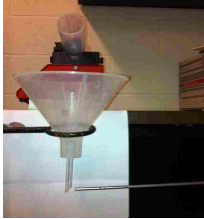
Figure 3.15. Setup of programmable motor (KD Scientific, KDS410) to determine the voltage reading of optical probes at different flow rates
