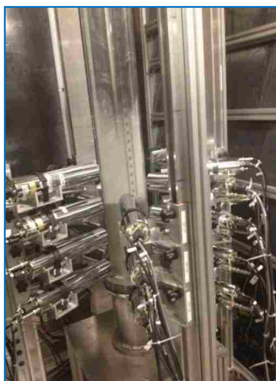
Figure C.1. a) Photograph of radioactive particle tracking (RPT) set-up and b) Top view of the detectors distribution for RPT Technique.
