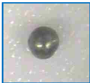
a)- Microscopic Picture of the Cobalt Particle (600 micron diameter)
