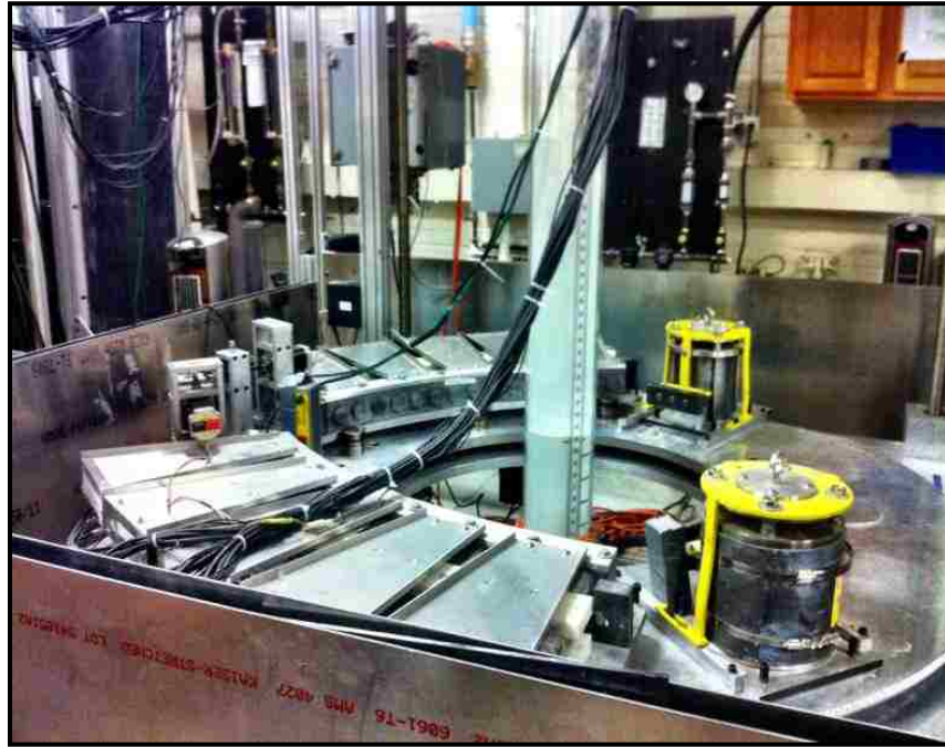
Figure 4.1 The photo of the single CT Setup with a 0.14 m fluidized bed reactor
