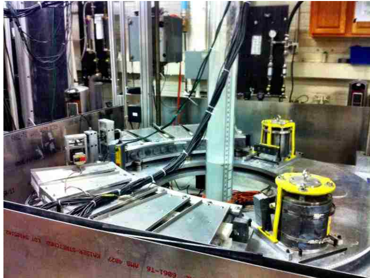
Figure B.1. The photo of the dual source CT Setup with a 0.14 m fluidized bed reactor
