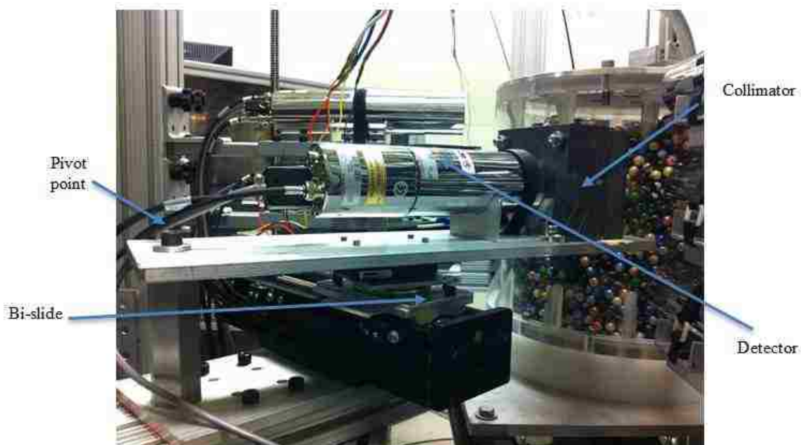
b. Side view of swinging collimated detectors I/II
