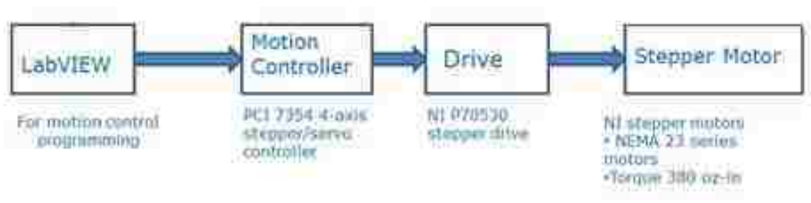
Figure 5.9 Block diagram of motion control system for swinging movement of the collimated detectors
