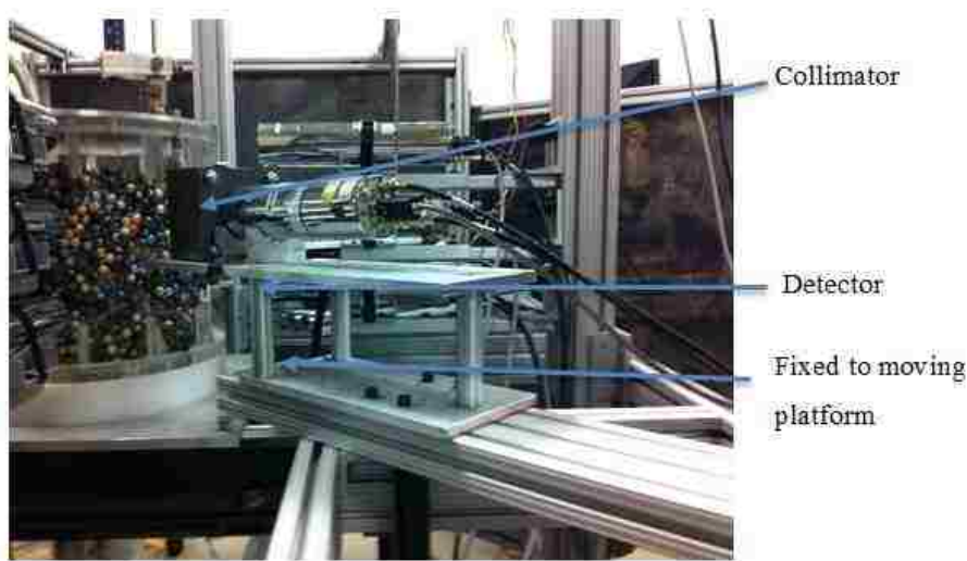
Figure 5.6 Collimated detector III having horizontal slit fixed to the moving platform
