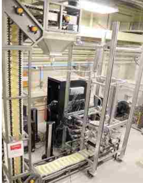
Figure 3.6 Continuous pebbles recirculation experimental set-up at Missouri S&T along with implementation of RPT technique
