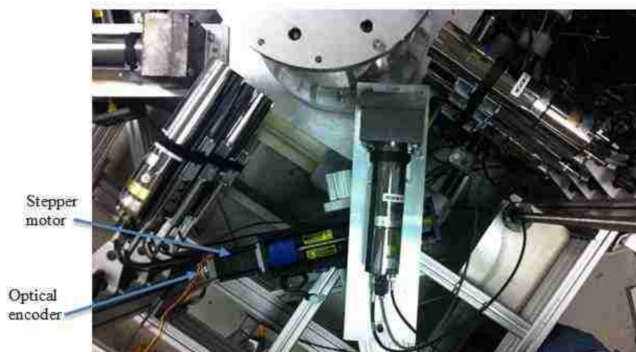
a. Top view of swinging collimated detectors I/II
