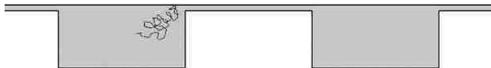
Figure 1. A 2D schematic view of an array of entropic traps. A DNA molecule in a wide channel is flowing into a narrow channel.
