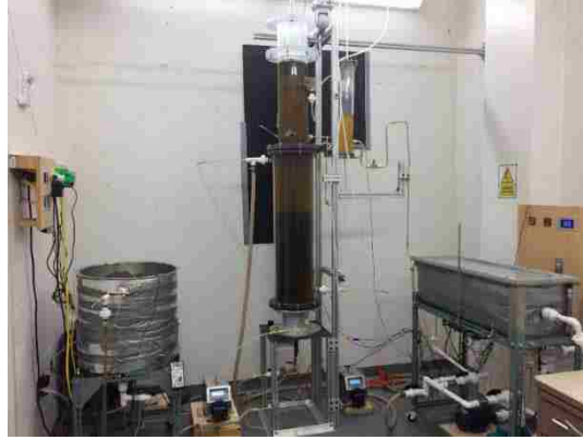
Figure 2. Two-stage anaerobic digestion process
