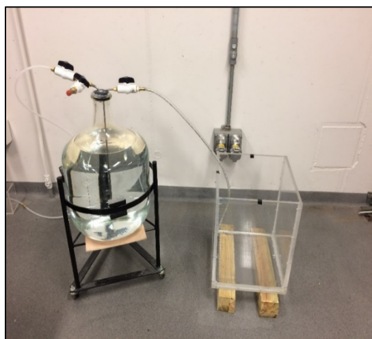
Figure 4. Biogas rate measurement by water displacement method
