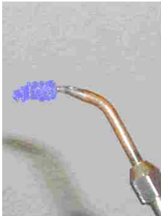
Figure 3. Flame Size and Shape for Flame Polishing.
