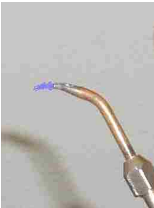
Figure 1. Size and Shape of Intense H 2 /O 2 Flame.
