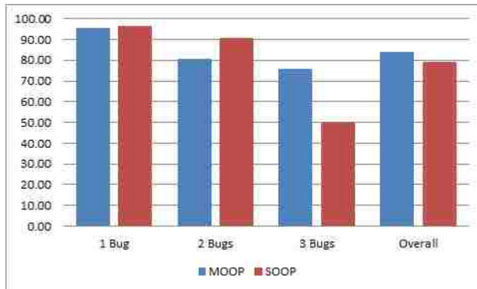
Figure 5.19: Percentage of Solutions Yielded in General Experiments that are True Solutions Ordered by Number of Bugs Present
