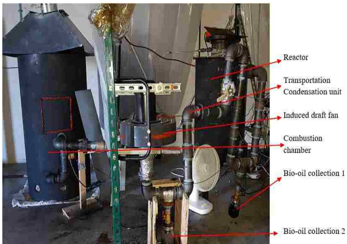
Figure 2.5. Complete gasifier system
