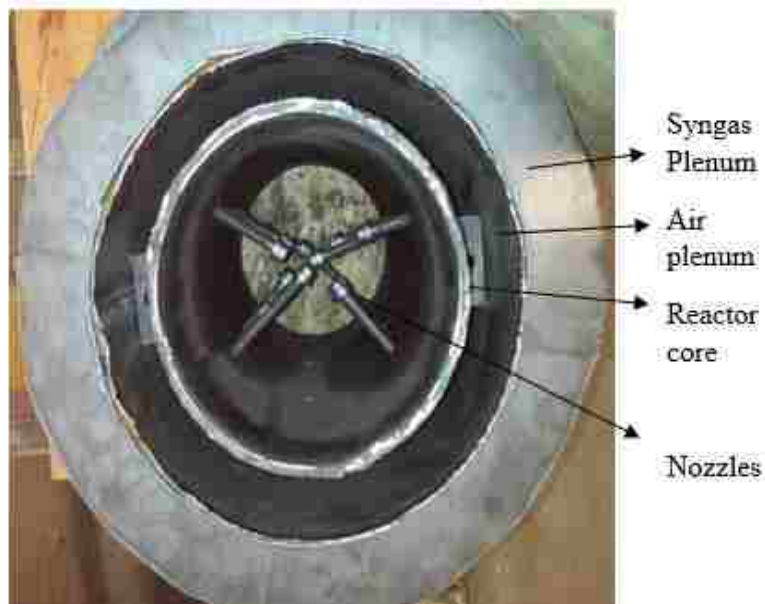
Figure 2.3. Assembly of air plenum and reactor core
