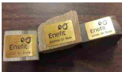
Figure 1.1. Left to right: Utah oil shale, Estonian oil shale, Jordan oil shale
