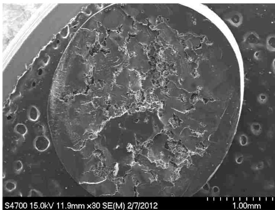
Figure 5.34. SEM of LLDPE-g-MA/93A sample (+ -) surface
