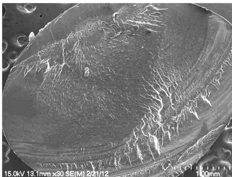
Figure 5.30. SEM of LLDPE/93A sample (+ -) surface
