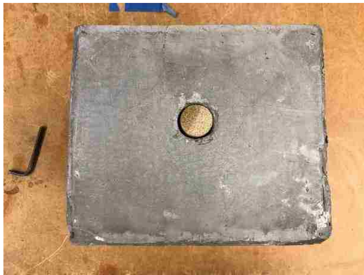
Figure 15. Paste sample with artificial defect (dowel).
