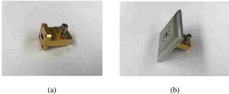
Figure 3. Open-ended waveguide probe with a standard (finite) flange (left), and a modified (engineered) flange (right).
