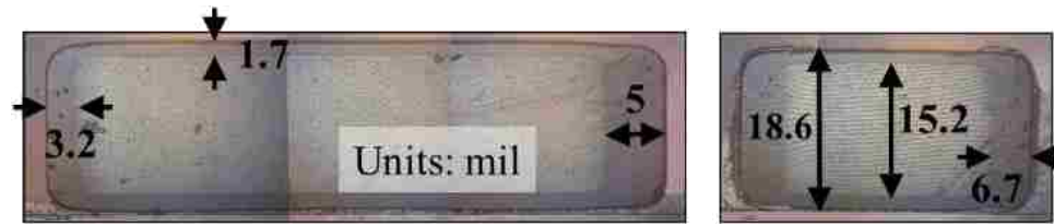
Figure 4. Cross-section of the divided 0603 capacitor under a microscope with 5x magnification [20].
