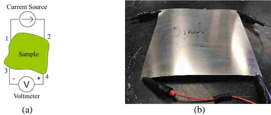
Figure 7. Test setup (a) schematic [15] and (b) sample under test for conductivity measurements.
