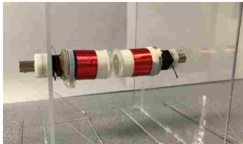
Figure 3. Air-core dual-loop magnetic field shielding test setup showing the air gap between the two loops used in the testing
