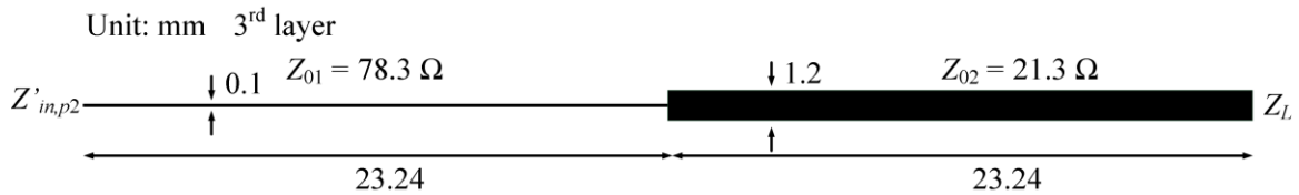
Figure 3.1. Dimensions of the two cascaded quarter-wave transformers in the third layer of the stack-up shown in Figure 2.1 (a).
